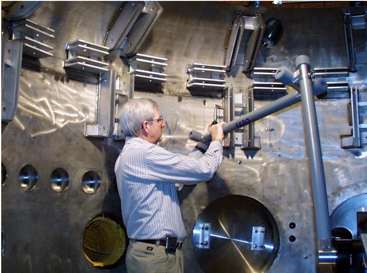
Figure 3-6 “Faro” Measuring Arm
