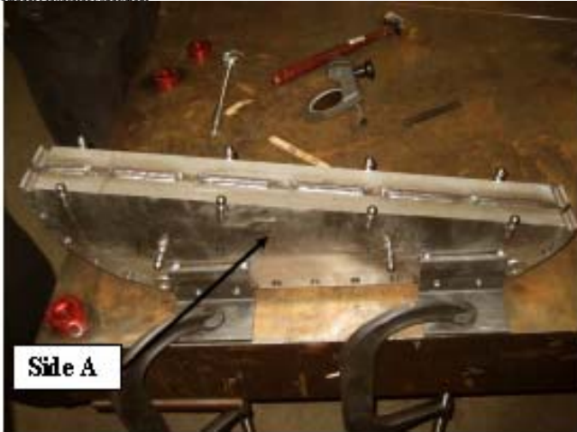
Phase I weld test specimen
