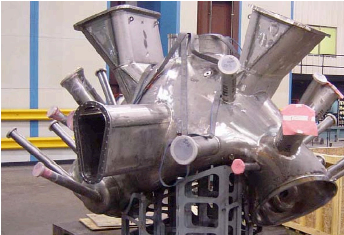
Figure 5(a). Vacuum vessel design. (b). Field period sector with ports installed for vacuum testing.
