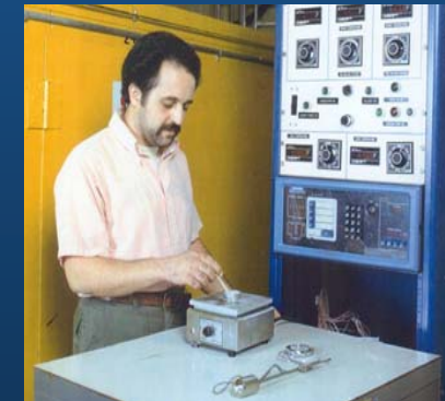
"Scrambled Egg" test to verify Gel temperature
