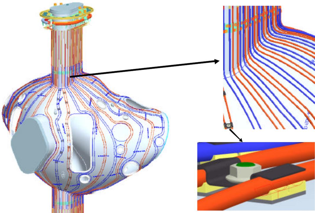
**Figure 1.0 Heating / Cooling Tube Arrangement**
