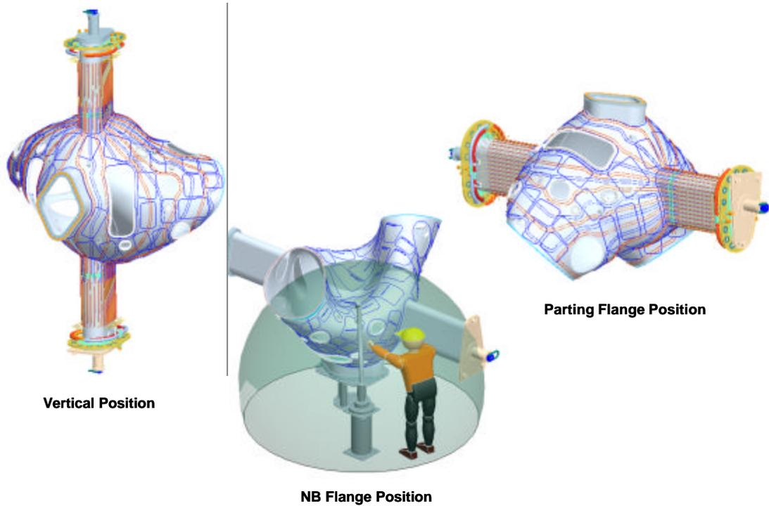
**Figure 3 Alternate Support Arrangements**
