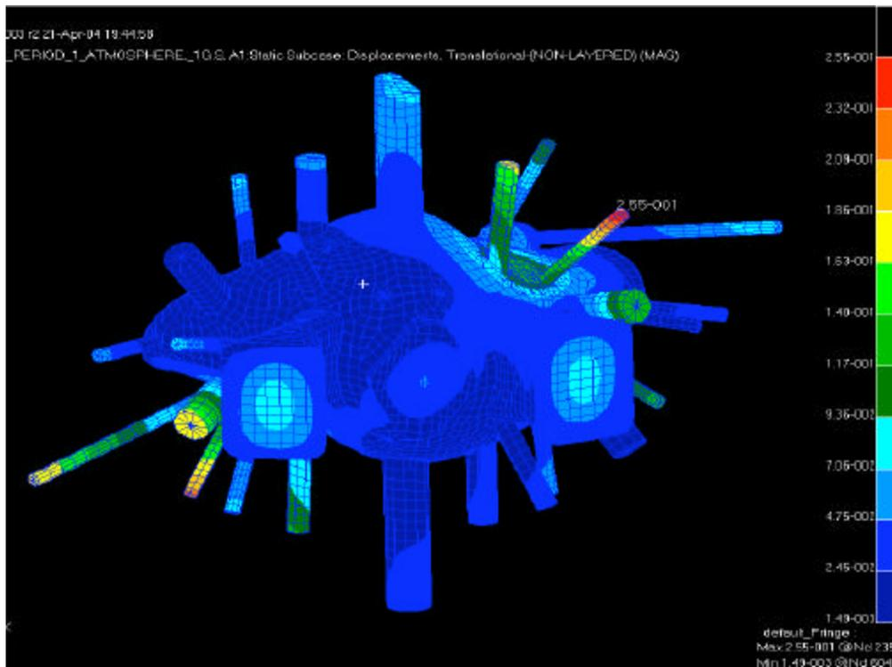
Figure 4 Vacuum Vessel displacement contours for atmospheric + gravity loads
