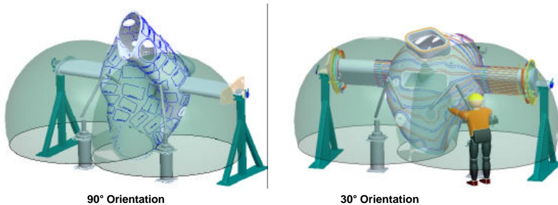
**Figure 2 Vertical port trunnion support arrangement**
