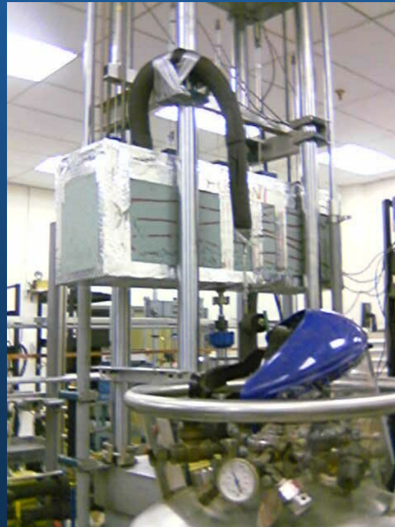
Sealed Insulation box with test bar Inside
