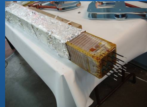
Bar Fitted with Probes for Electrical Testing after Cycling
