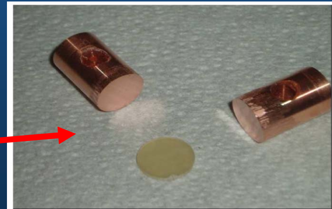
Figure 5. Typical adhesion to metal surface failure.
