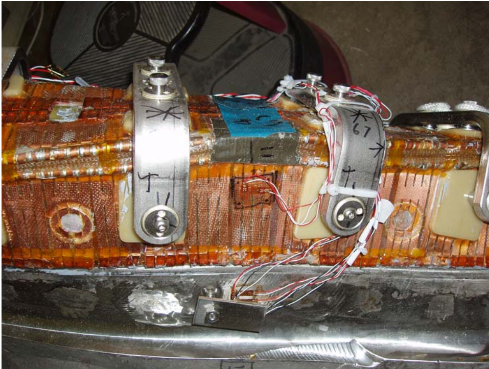
Figure 5-34 Strain gages at Clamp 68 - Side B
