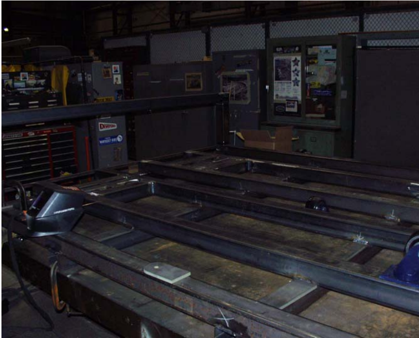
Figure 5-24 Cryostat carriage in fabrication
