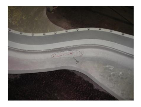
Group 5 is a cluster of indications on the datum D side in radius below VPI groove between T holes 8 and 11. The longest indication is a .7" linear.
