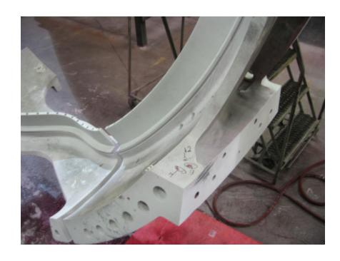
Indications 12, 13 and 14 are a group of indications located on the large cutout on the datum D side between flange holes 4 and 5.
