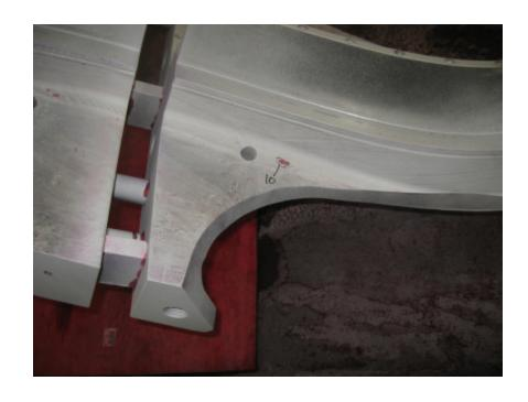
Indication 10 is a .700" linear located in the radius below the VPI groove on the datum E side between T holes 13 and 14.
