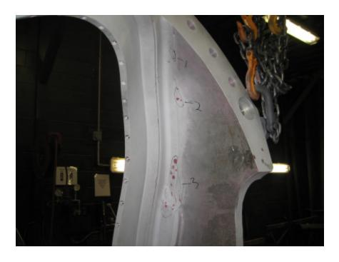
Group1is a small cluster of linear indications, longest is .5". Cluster is located in the radius below the VPI groove on the datum D side between T holes 43 and 45.
