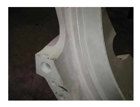
Indication 6 is a .400" linear located in large cutout of datum D flange between flange holes 16 and 17.
