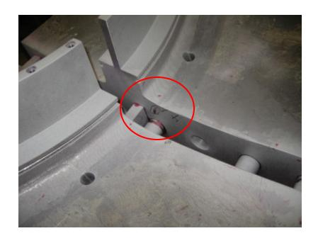
Indication 4 is a 1.5" linear located on the poloidal break (datum D side).
