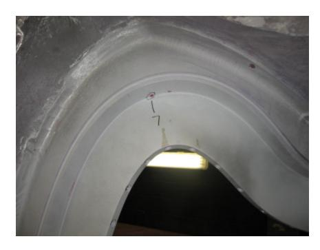
Indication 7 is a .15" rounded between T holes 77 and 78 on the datum D side.
