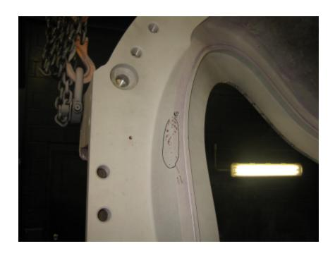
Group 11 is a cluster of indications on the small outer wing surface on the datum E side. Largest indication is a .700" linear.
