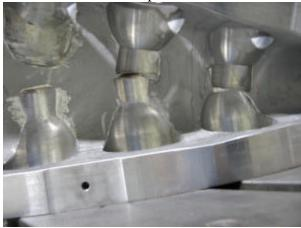
3. Poloidal Break, Datum D side. Casting radius between T section and inner wall extends beyond the G11 shim approximately .300" on each side.
