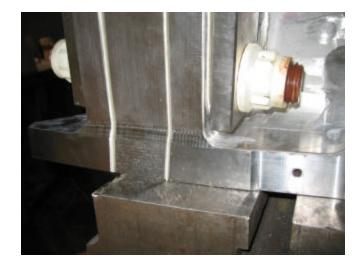
G11 shim has a full radius on both ends. The drawing shown below shows only the radius toward the inside cast wall.
