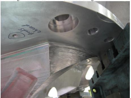
7. Various tool cutter marks on the D side short leg between holes 34 and 42. Cutter marks are no deeper than .010".
