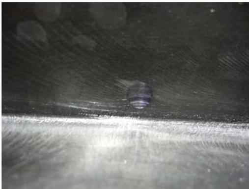
Round tool mark on short leg E side of T section. Mark is approx. .200" round and .010" deep.
