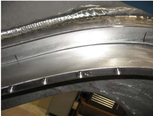
Tool marks on short leg of T E datum side between holes 8 and 12. The tool marks are less than .005" deep.
