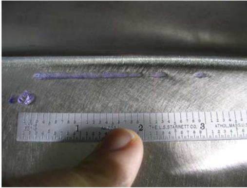
Tool gouges on long leg of T E datum side between holes 6 and 7. Gouges are approx. 3" long and .005' deep.
