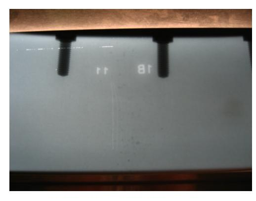
View above is of a cluster of porosity between holes 43 and 44. The largest was sized at approximately .090".
