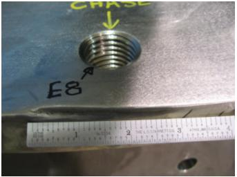
8. The pictures below are of the flange holes repaired under NC20449. There is no nonconforming condition to report but I felt this was worthy of documenting.
