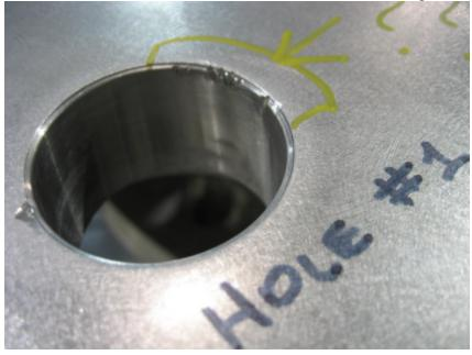
6. Groove in the 1.885 thru hole located at D flange hole 18. The groove is approx. .018" deep x .400" wide and is visible on 50% on the diameter.
