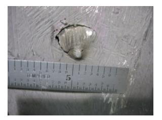
2. Small tooling gouge on long leg of T on D side near hole 33. Gouge is approx. .120" x .08" and less than .010" deep.
