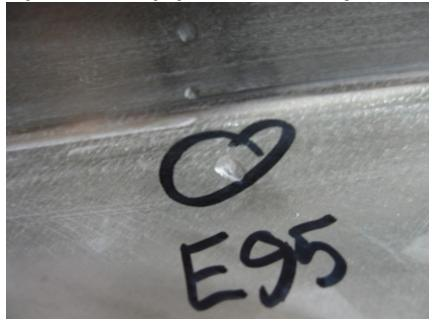
10. Tool gouge located on short leg of T near hole 77 on E datum side.
