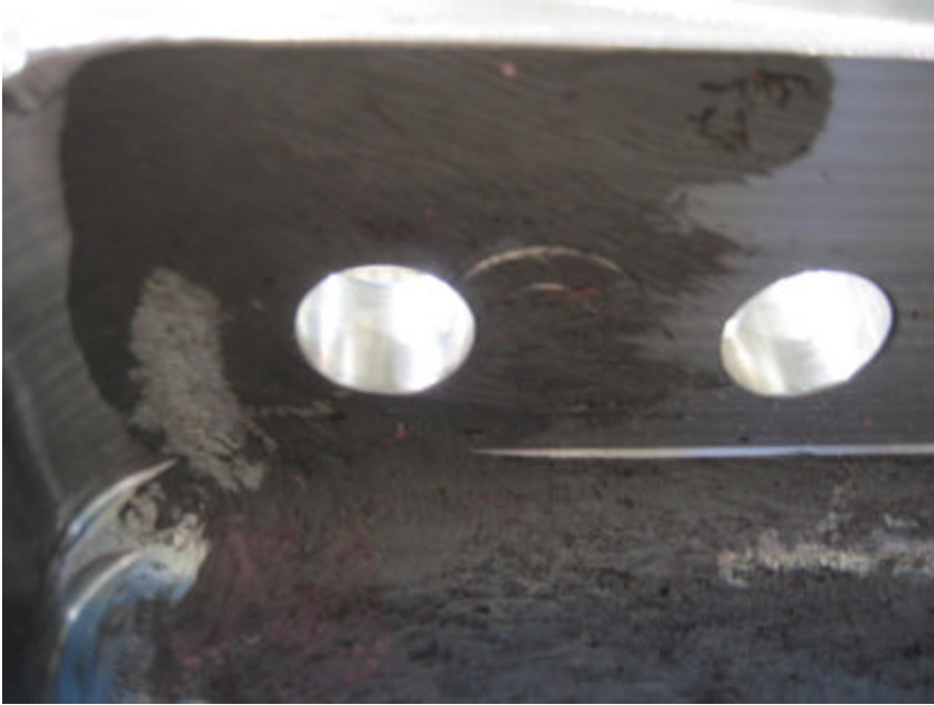
Noncleanup of foot on back side of D flange.JPG
