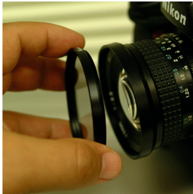
1. Screw ND filter to lens barrel
