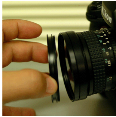
2. Screw strobe ring into ND filter.
