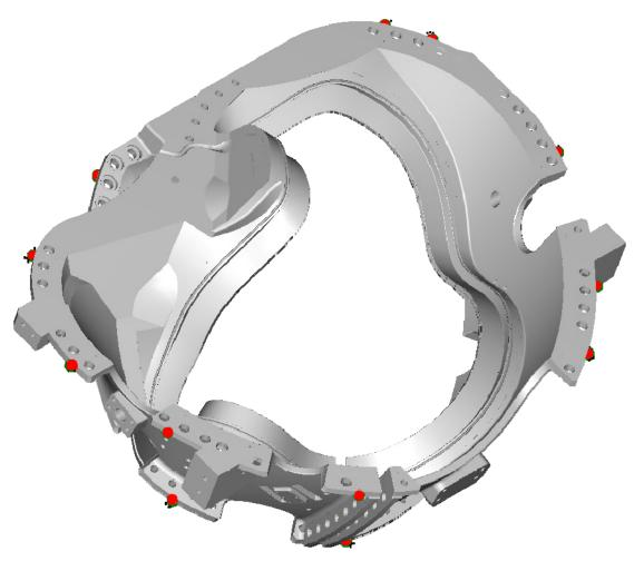
MTM flange tooling balls used for initial inspection and alignment
