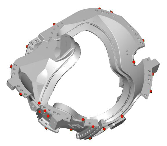
After winding, metrology transitions back to flange tooling ball locations and adds body tooling balls
