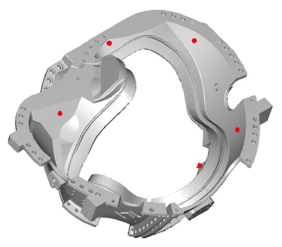
PPPL adds 15mm conical seats for subsequent alignment during winding
