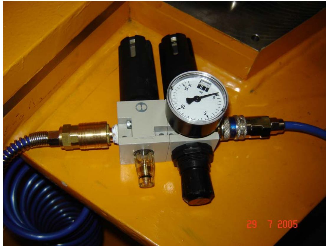
THE PRESSURE REGULATOR ( p= 3,5 bar) FOR THE PNEUMATIC CARTRIDGE SQUEEZING MACHINE
