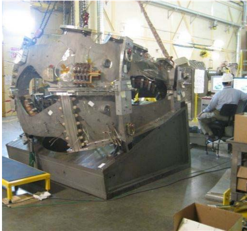
Figure 2.4-2 Mating “B” Coil into Position
