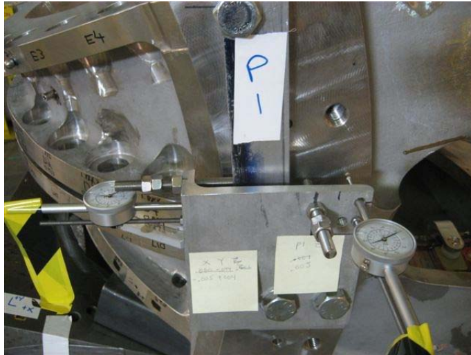
Figure 2.4-3 Jack Screws and Dial Indicator Installation
