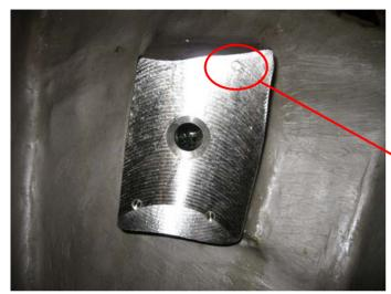
The 3 hole pattern would be shifted .25" (parallel to the datum E flange) to accommodate the hole circled in the pattern above.
