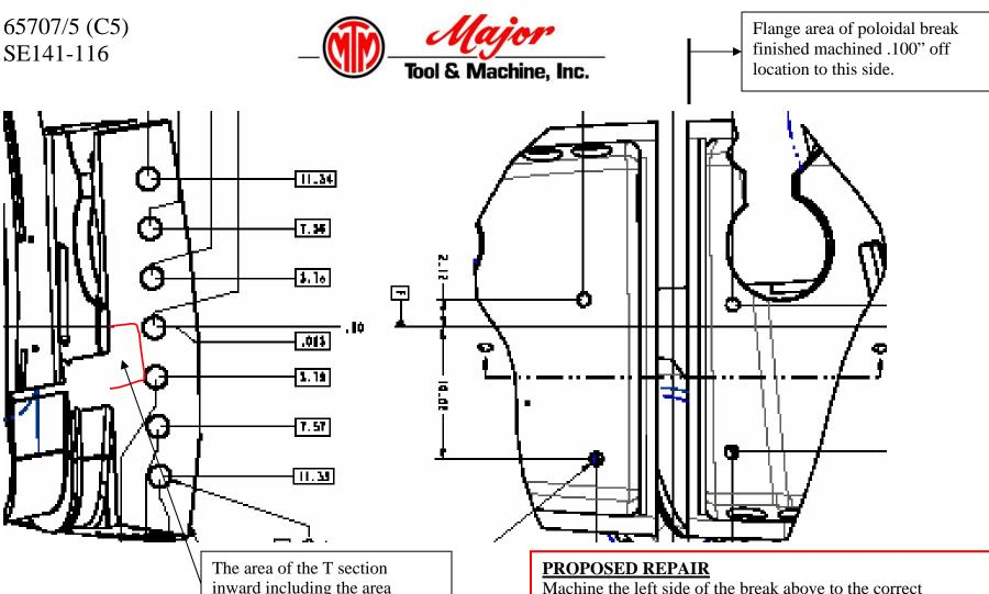
The area of the T section inward including the area highlight in red has been undercut into this surface approximately .08". This area has been cut on location.
