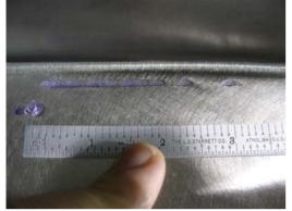
Tool gouges on long leg of T E datum side between holes 6 and 7. Gouges are approx. 3" long and .005' deep.
