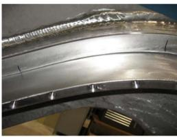
Tool marks on short leg of T E datum side between holes 8 and 12. The tool marks are less than .005" deep.
