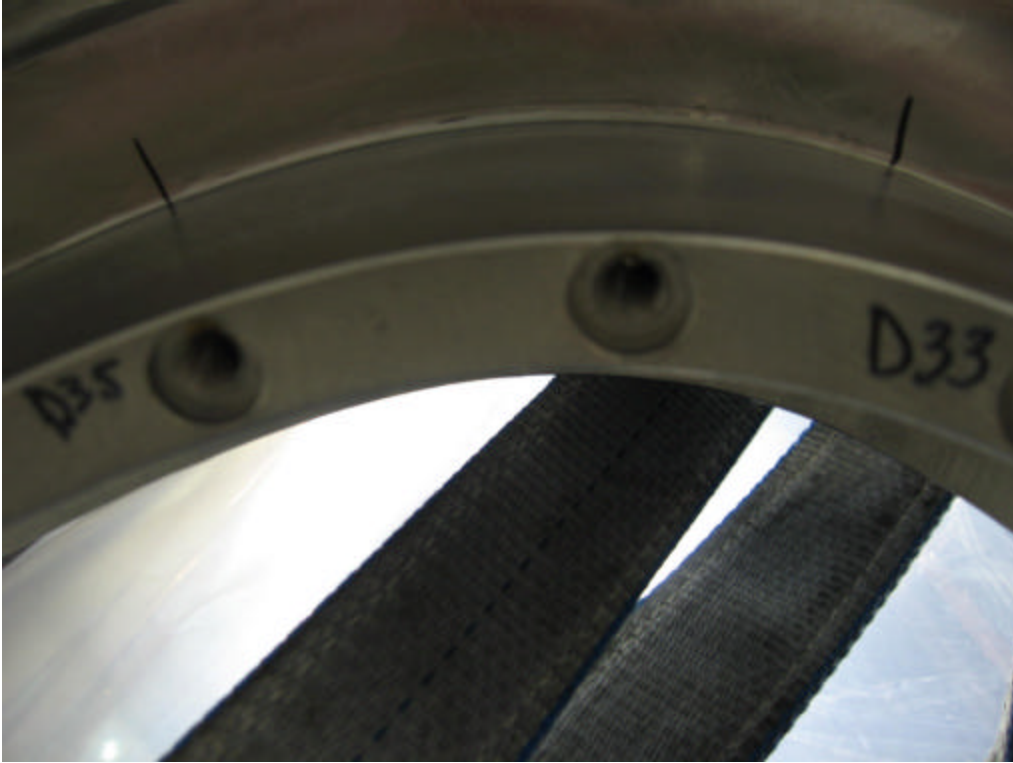
Area of cutter noncleanup near radius between D33 and D35. Approx. .008" max depth.
