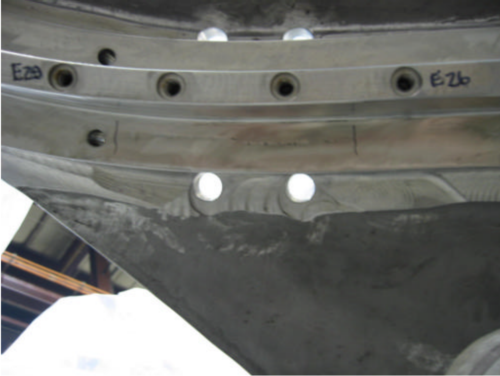
Wide view of cutter noncleanup on short leg between holes 26 and 29 on E side.
