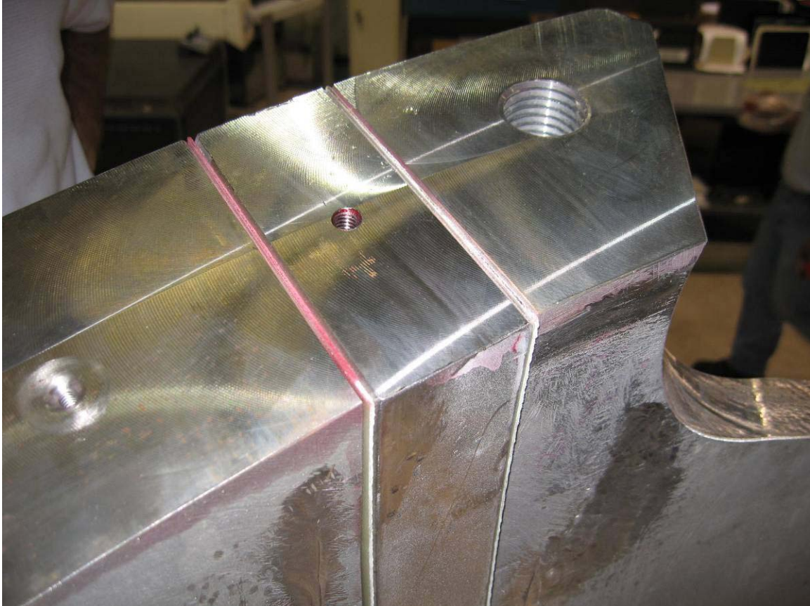
Penetrant on G-11. Break has not yet been tested electrically.
