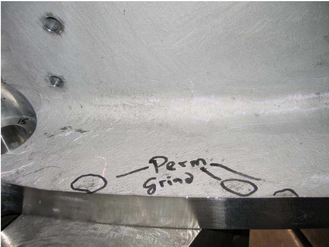
VPI groove looks good other than this one spot already identified.
