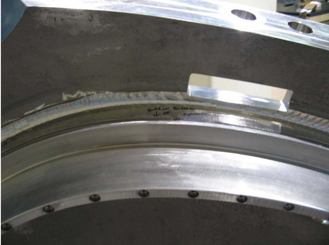
VPI groove looks good other than this one spot already identified.
