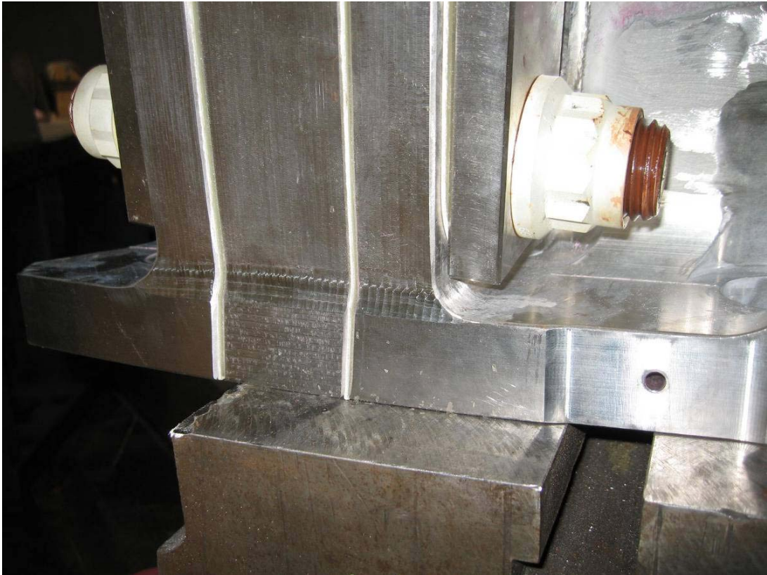
Poloidal Break Fit-Up. Significant gaps where machined-to-print G-11 does not match machined-to-contour Shim.
