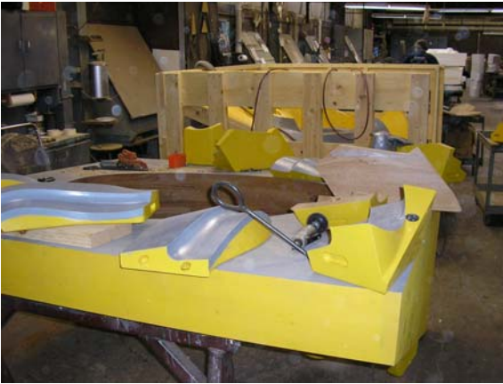
Top of the drag box - loose piece.
