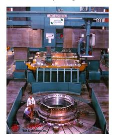
DORRIES SCHARMANN Traversing Gantry milling and boring Center Maximum part length 20 meters (65.5 ft.), maximum part width 6.6 meters (21.6 ft), maximum part height 5 meters (196 inches), VTL table 6 meters (19.6 feet),
