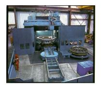
Berthiez TDM 250 - Maximum part diameter of 168", maximum part height of 127", pallet changer, 2 live spindles, grinding attachment, swiveling indexing head, tool probe, part probe, G.E. Fanuc 15, 135 HP table motor.
