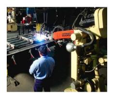
Motoman Welding Robots compliment our automated welding abilities. One robot features pulsed metal arc welding and high definition plasma cutting. The features plasma arc welding used in conjunction with automatic seam tracking. Five weld positioners are utilized in conjunction with the two units.
