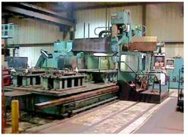
Sera Mill Vertical Gantry Machining
