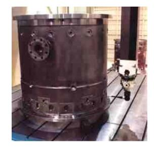
In addition to our coordinate measuring machines, we utilize tool and part probing on our machine tools to take readings during production. Probe data can then be imported directly into our manufacturing system.
