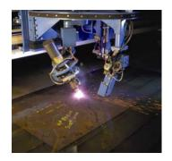
The Burnout Table is equipped with a nesting program to maximize material by laying out the best burn pattern for the needed part vs. the available plate material.
