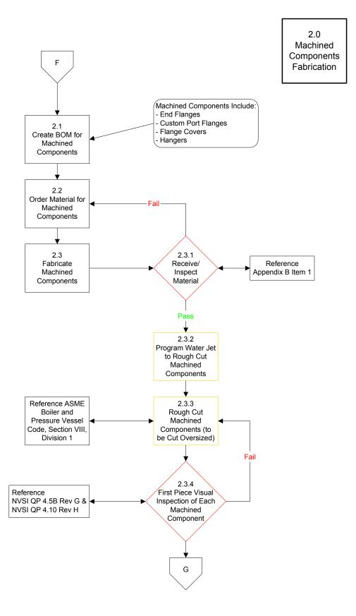
2.0 Machined Components Fabrication
