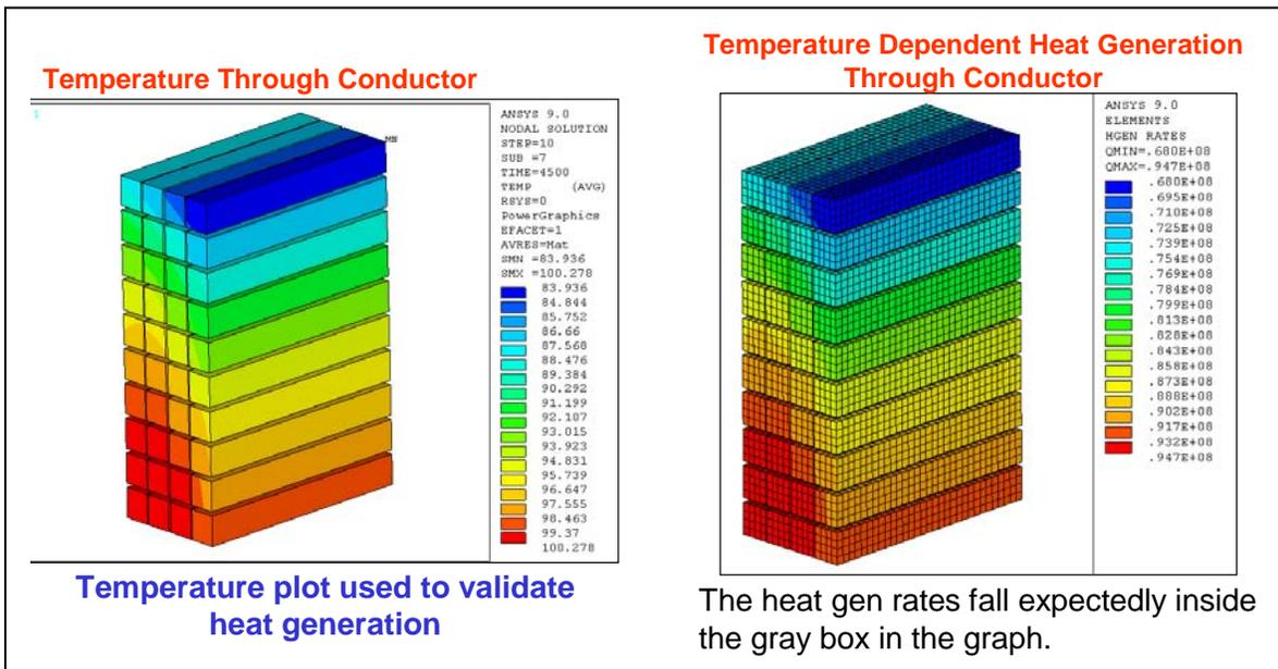
Figure 16: Test Case for Heat-Temperature Dependency
