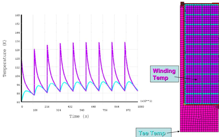
Figure 22: Ratcheting of modular coil and tee (20 Minutes)
