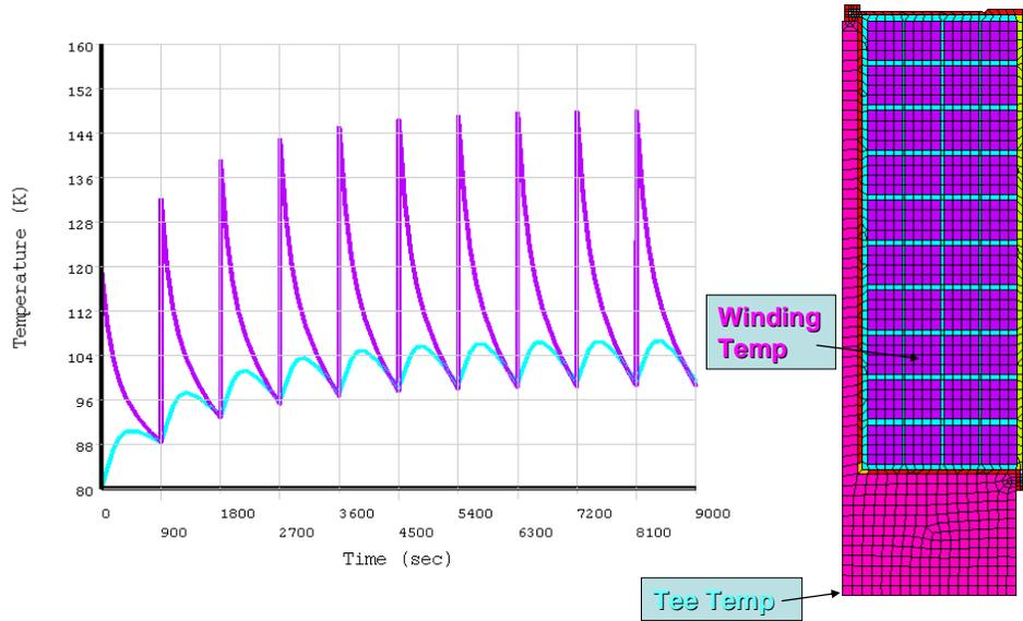
**Figure 19: Temperatures ratcheting for a 15 minute cool down period**
