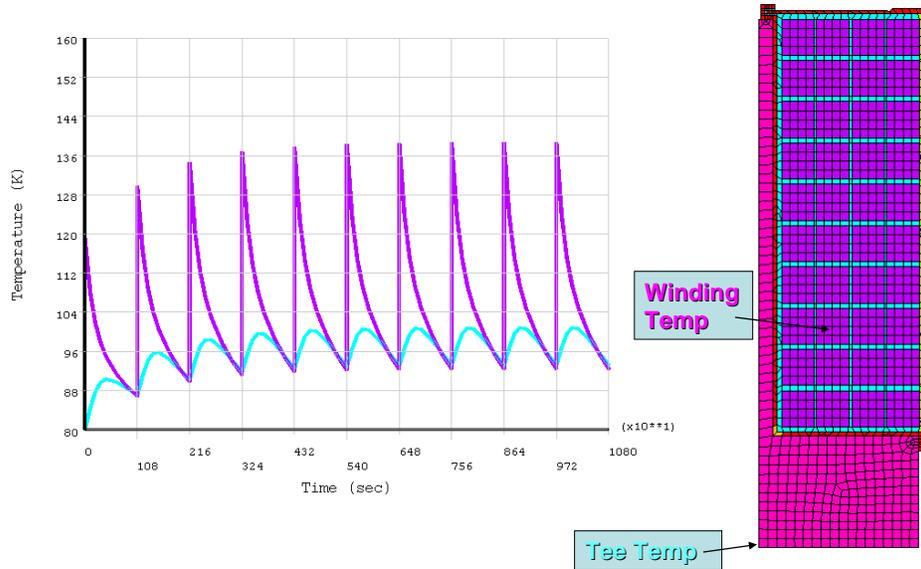
Figure 21: Ratcheting of modular coil and tee (18 Minutes)
