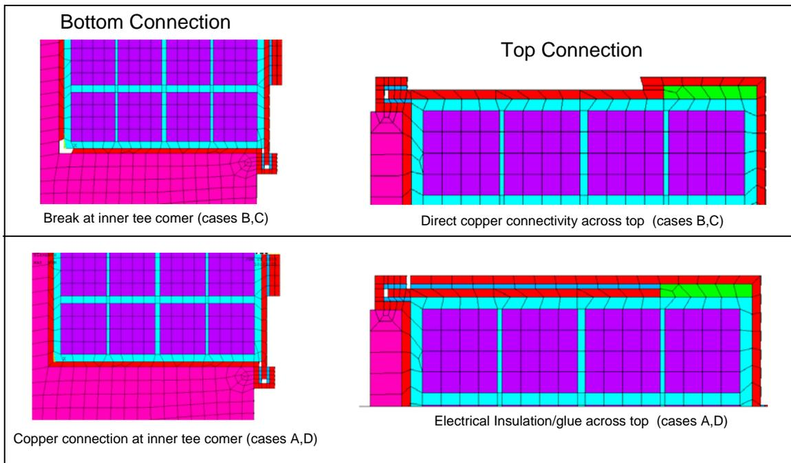
**Figure 2: Cladding connection configurations, upper insulation alternatives.**
