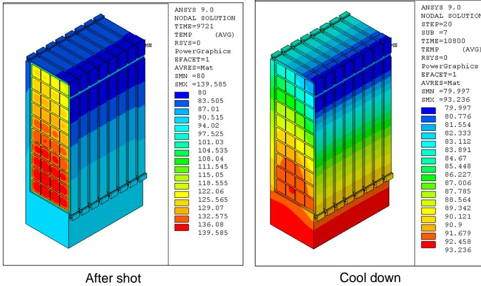
**Figure 20: Last pulse/cooling period with 18 minute cool down**
