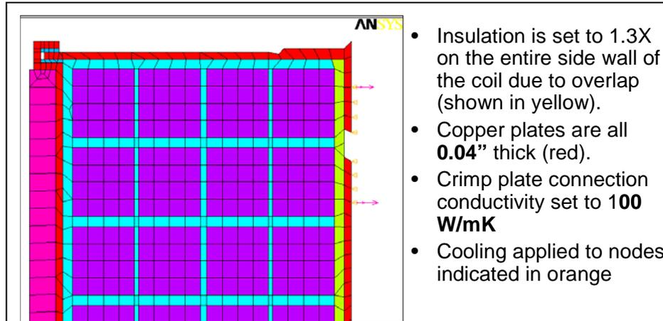
**Figure 14: Cross sectional view of alternative two tube configuration.**
