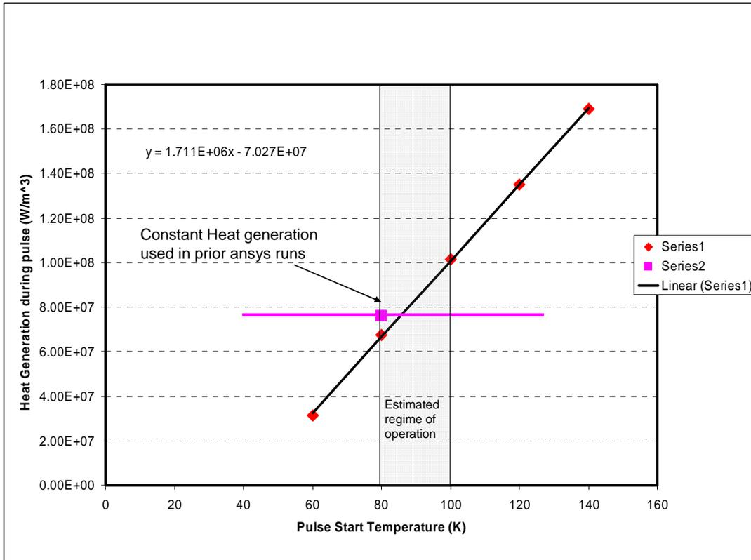
Figure 15: Average heat generation rate as a function of temperature.
