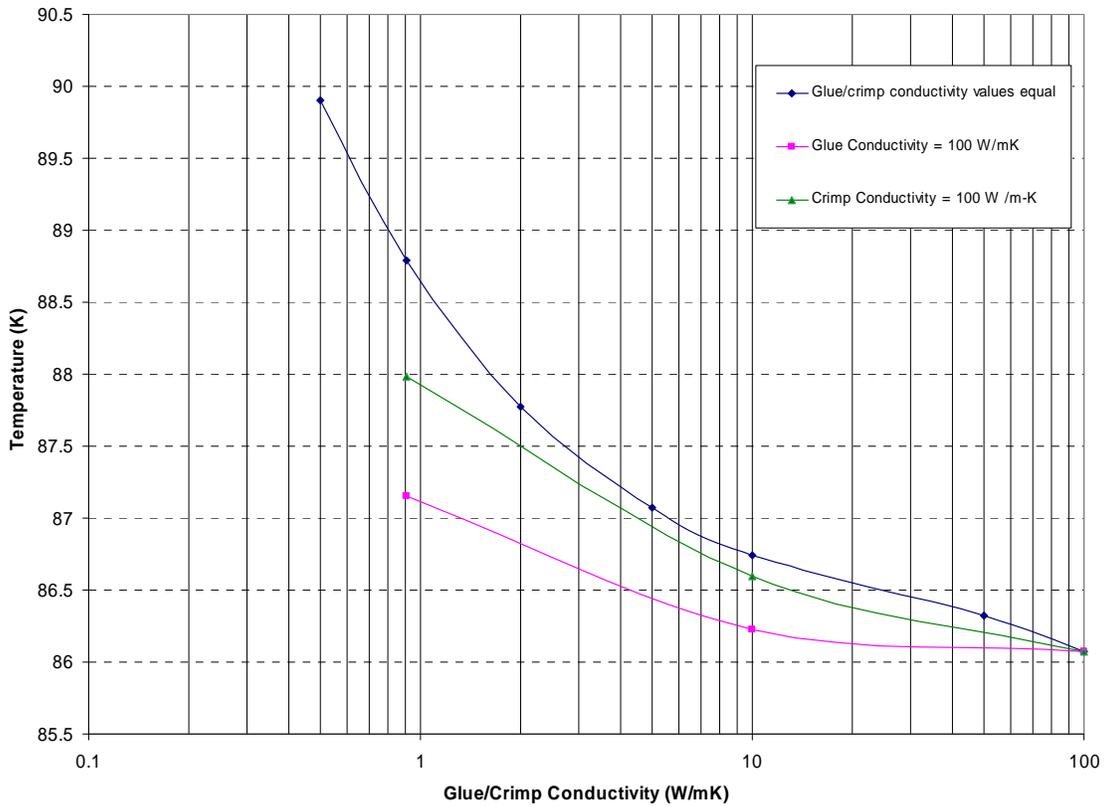
Figure 12: Crimp/glue conductivity dependency on log scale
