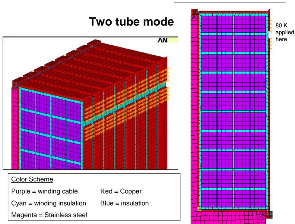
**Figure 13: Alternative 3d view of geometry and mesh for two tube configuration**
