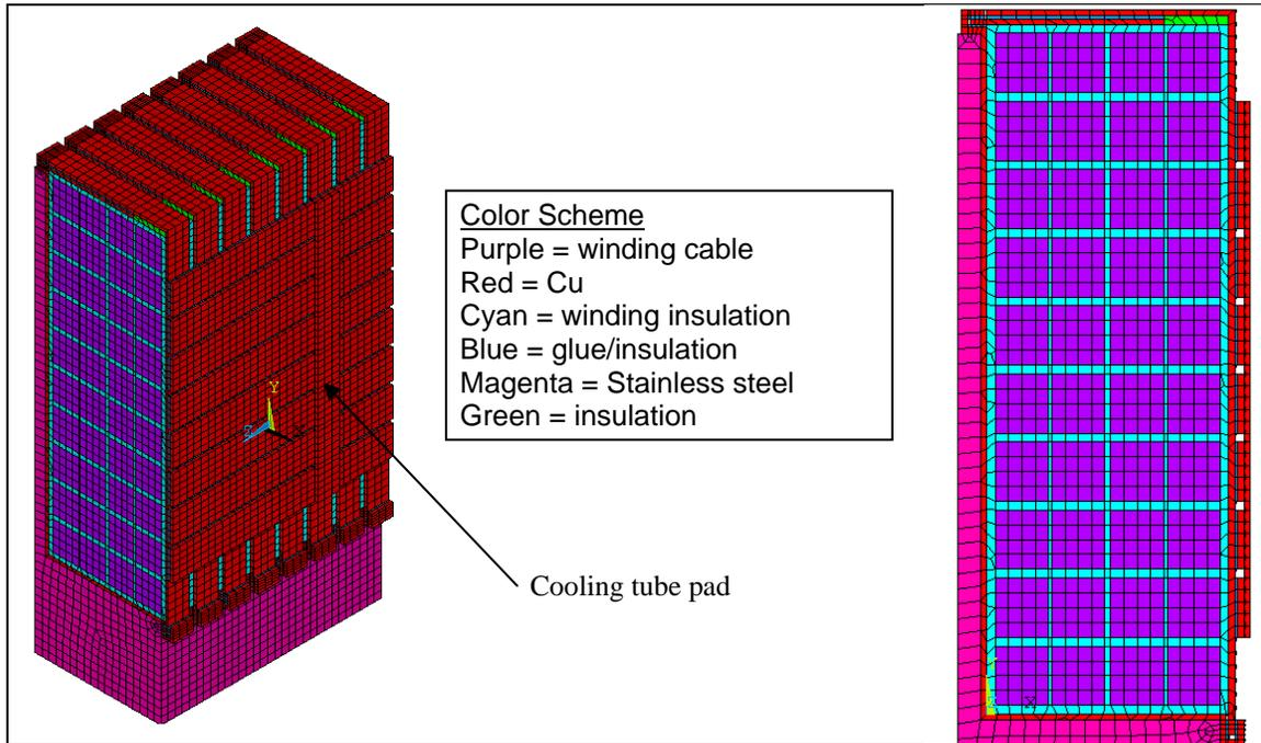
**Figure 1: Mesh used to model winding pack section**
