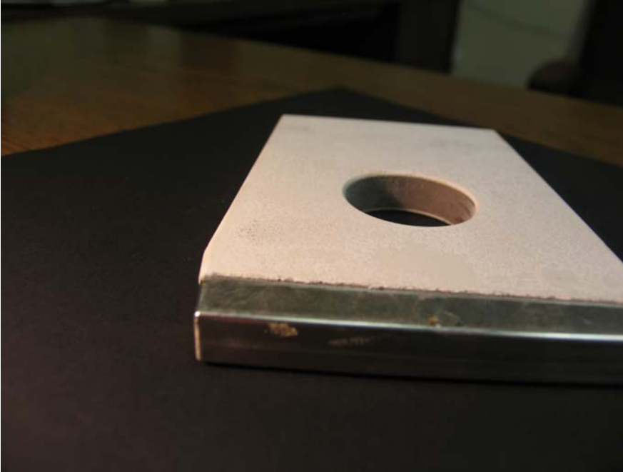
Shim after cycling test, showing “quilted” pattern on alumina.
