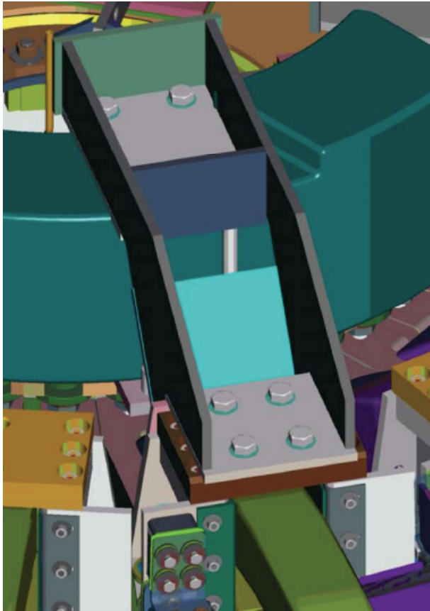
Figure 2a. PF-4 coil supports
