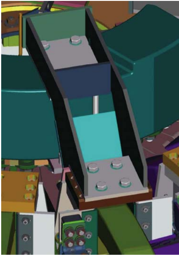
Figure 2a. PF-4 coil supports
