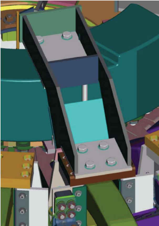
Figure 2a. PF-4 coil supports
