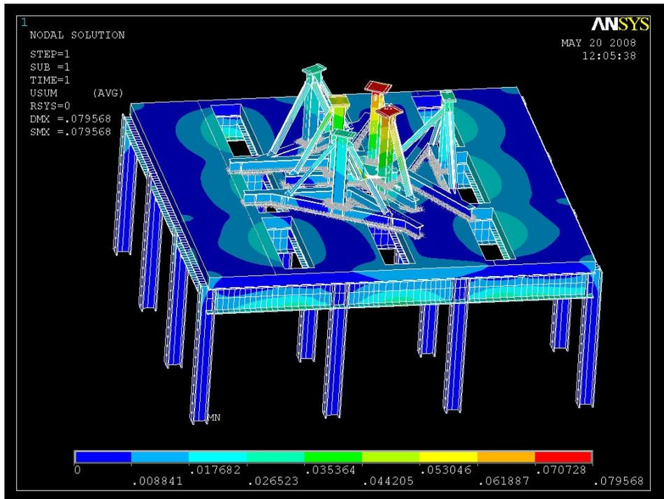
Figure 11 - SRSS Displacement contours of base supports – Load Case 2
