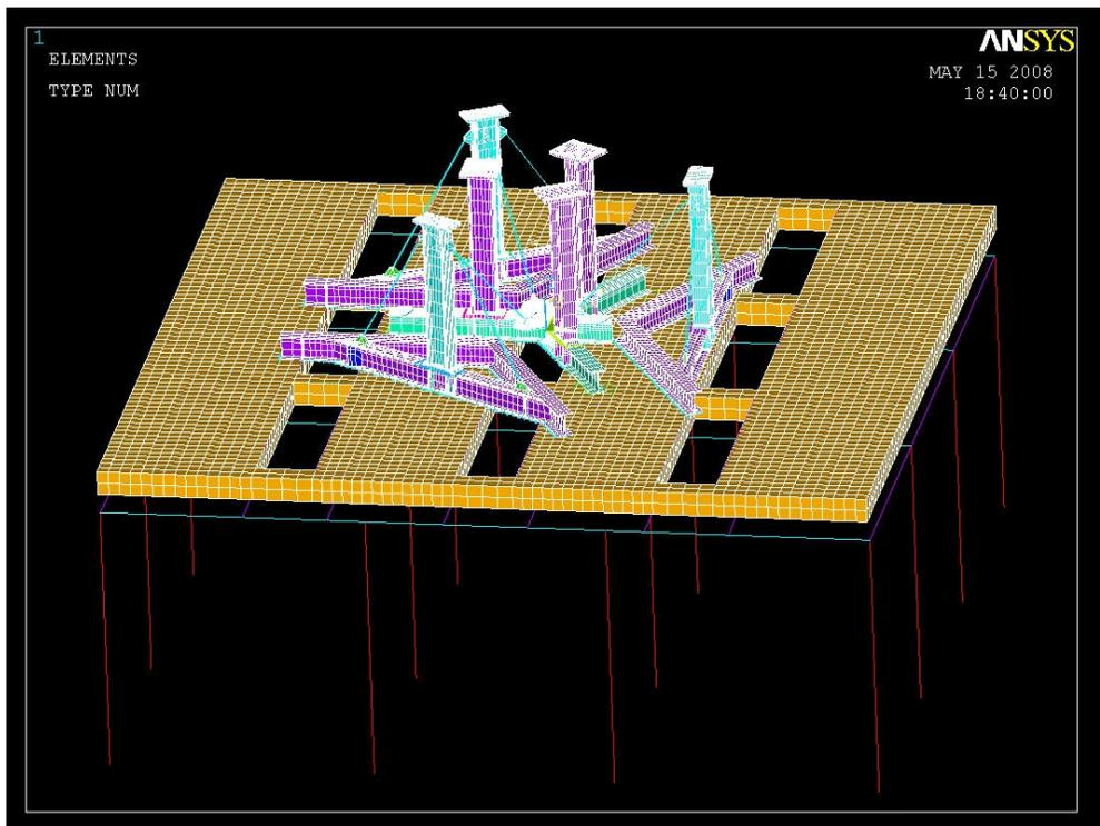
Figure 3 - ANSYS FEA Model of the Base Supports & Test Cell Floor (full-base-supt-model-F4h)
