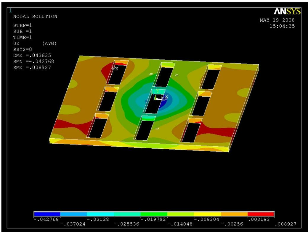
Figure 6 - Test Cell Floor Vertical (dz) displacement contours -stellarator core at room temperature
