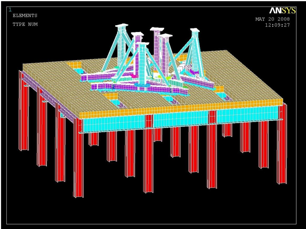
Figure 8 - Re-modeled floor girders & stringers (full-base-suppt-model-F4j)
