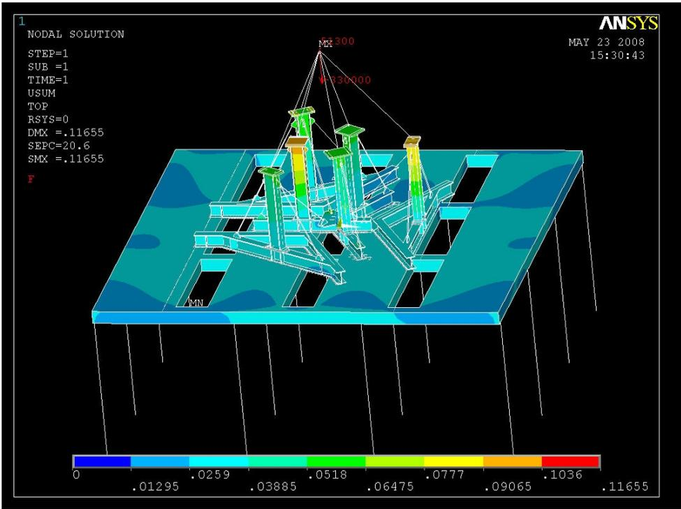
Figure 16 - SRSS Displacements for north-south seismic loading condition
