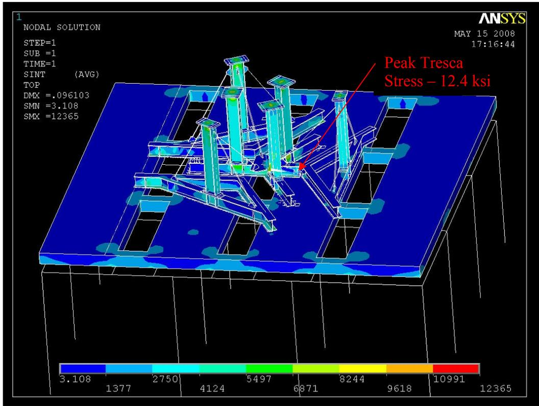
**Figure 7 - Tresca stress contours -stellarator core at room temperature -peak stress is 12.4 ksi**
