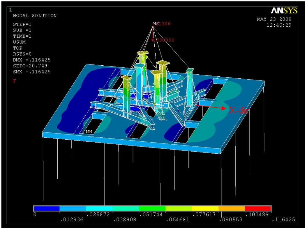
Figure 14 - SRSS Displacements due to an east-west static seismic loading condition
