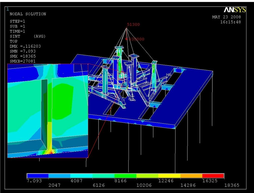
Figure 17 - Tresca Stress contours for north-south seismic loading condition
