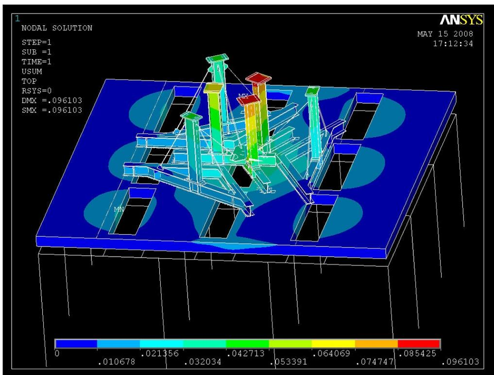
Figure 4 - SRSS Displacements due to gravity loading –Stellarator core at room temperature
