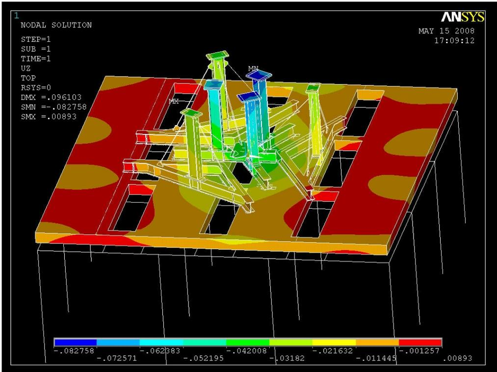
Figure 5 - Vertical (dz) displacement contours -stellarator core at room temperature
