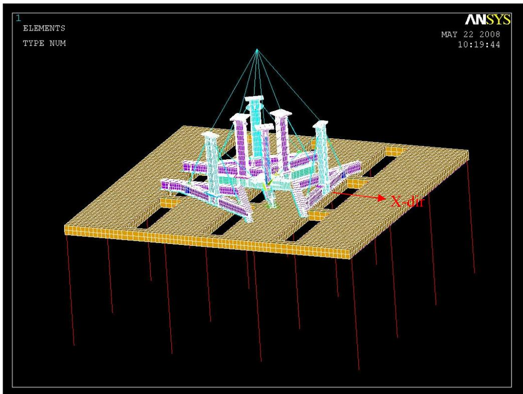
Figure 13 - Seismic model of NCSX machine base supports
