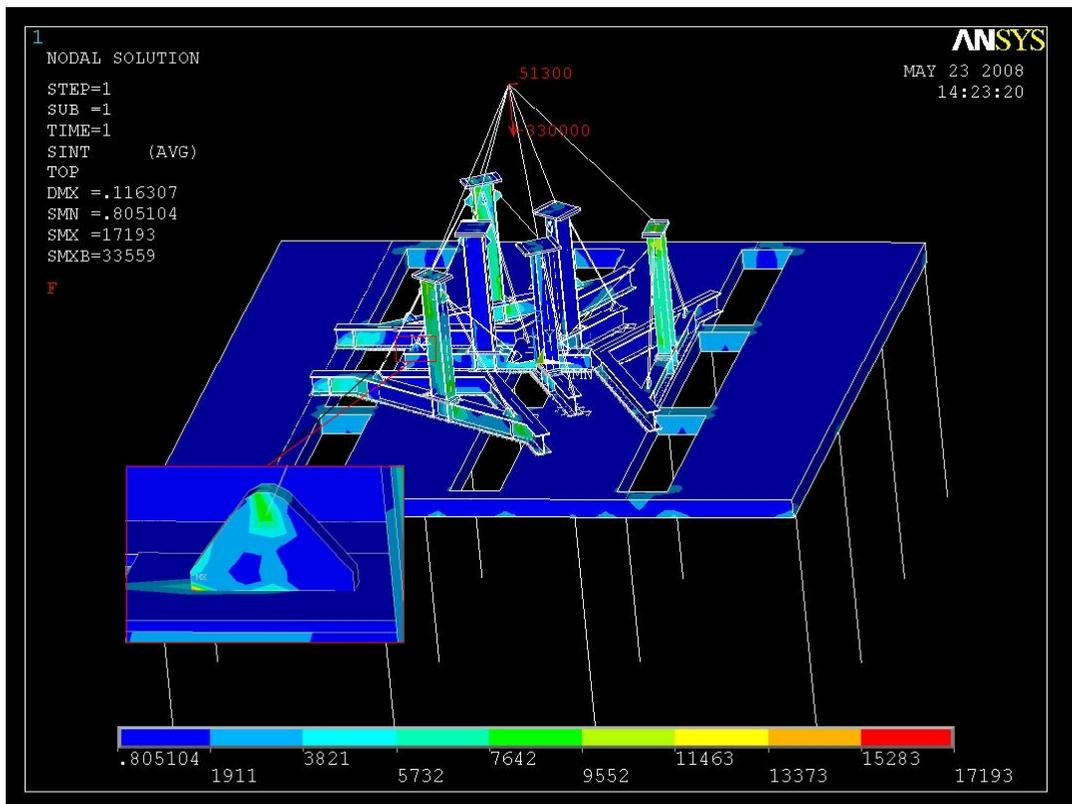
Figure 15 - Tresca Stress contours due to east-west seismic loading condition
