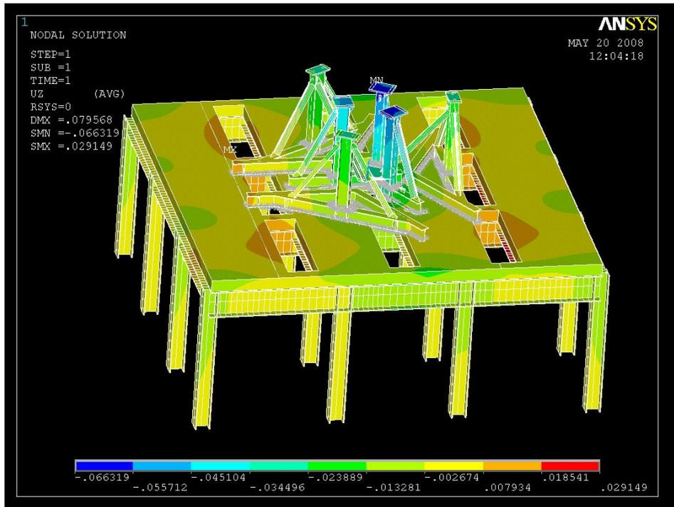
Figure 10 - Vertical displacements of the base support structure – Load Case 2
