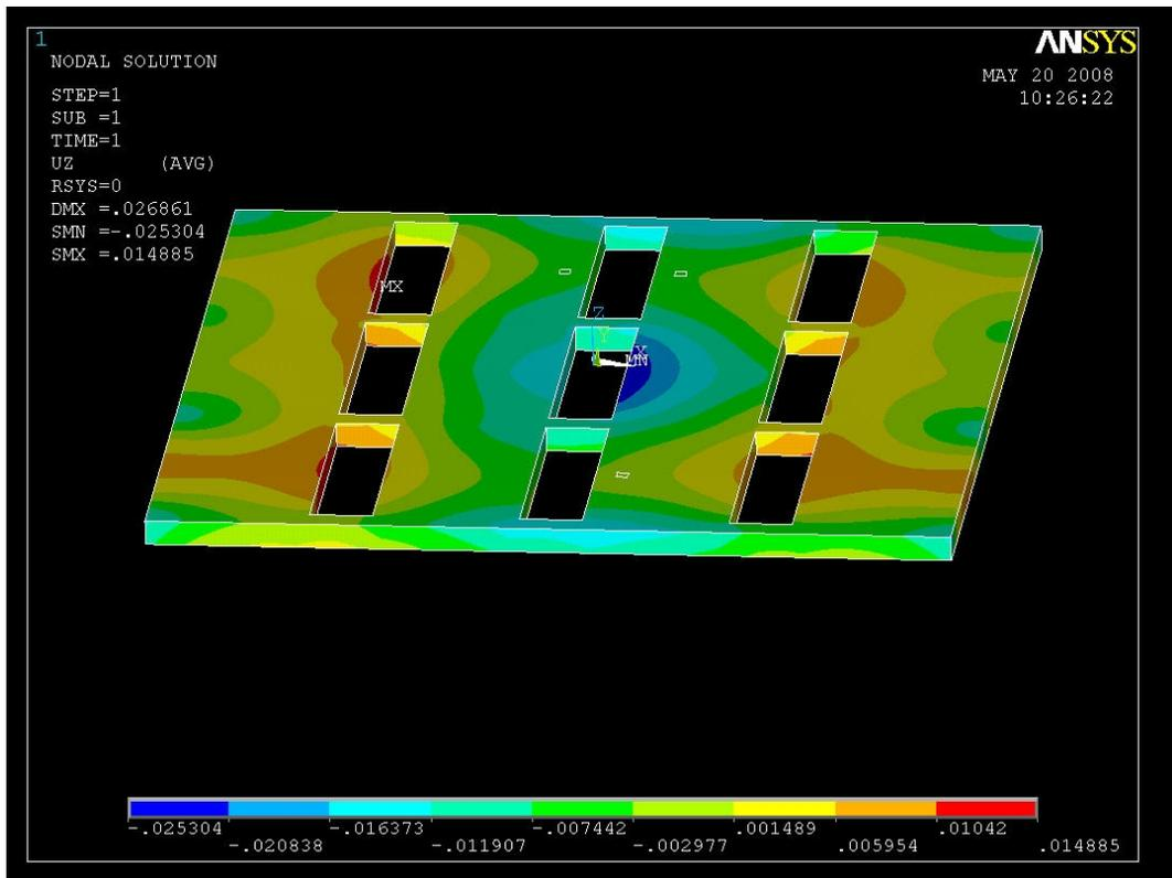
Figure 9 - Vertical displacements of the test cell floor – Load Case 2
