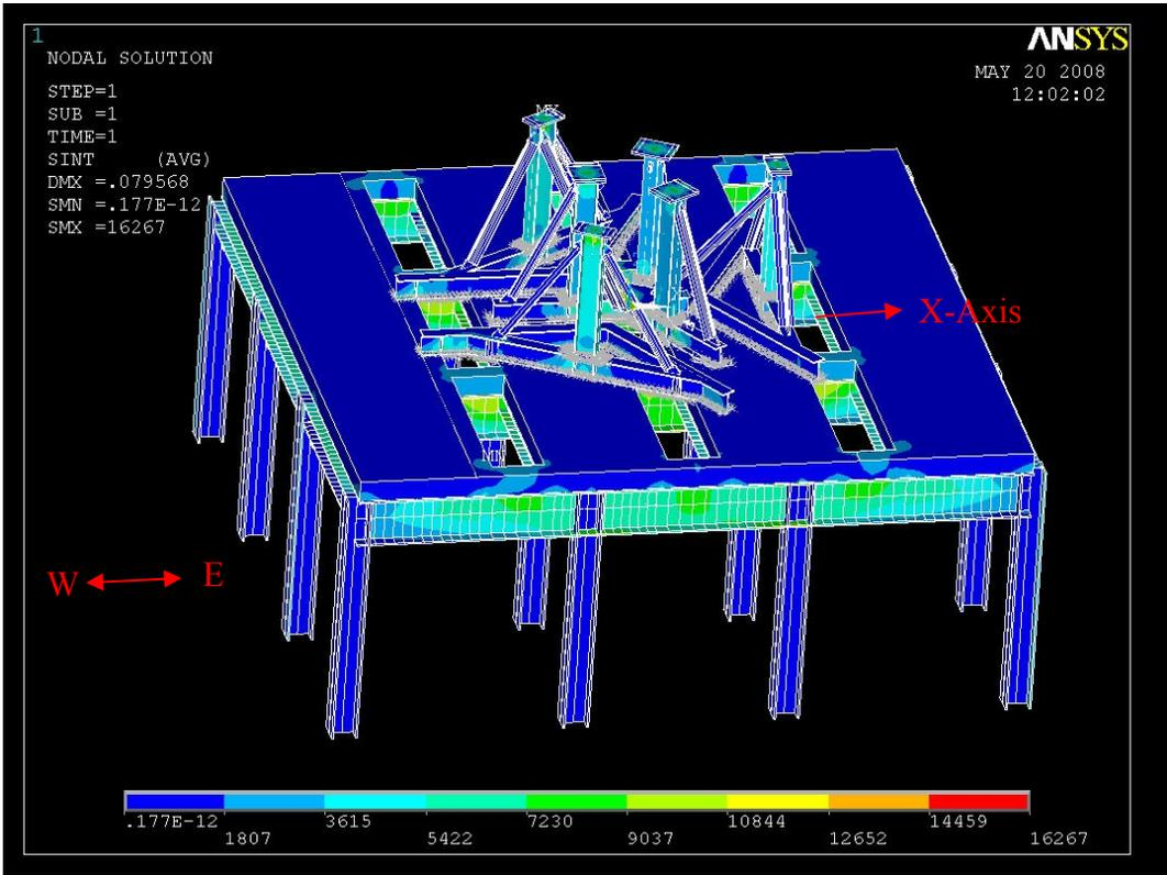
Figure 12 - Tresca Stress contours for Load Case 2
