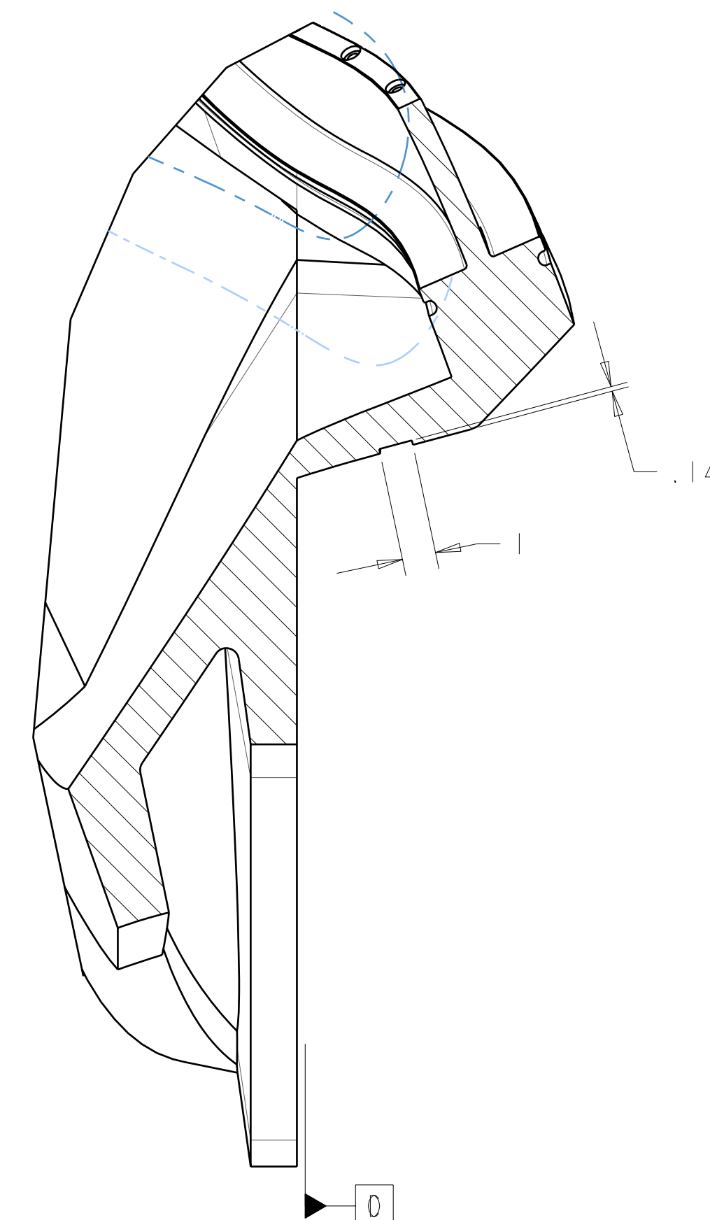
SECTION W-W WING SHIM POCKET SCALE 0.25
