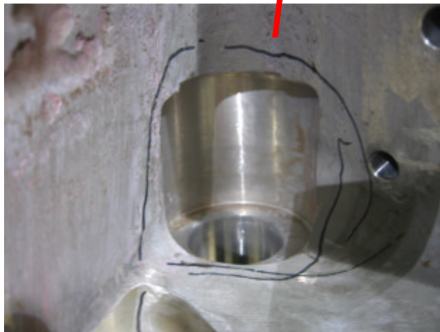
Picture to the left is of the 3" counterbore in the datum E flange as reported on NC21252 step 810. Area shows heavy stock around hole (too much to grind).
