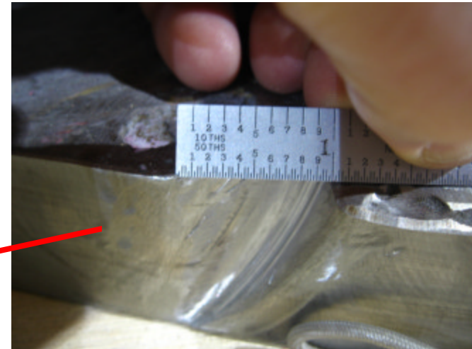
Tool Gouge on perimeter of Datum E flange, approximately 1" wide by .50" deep.
