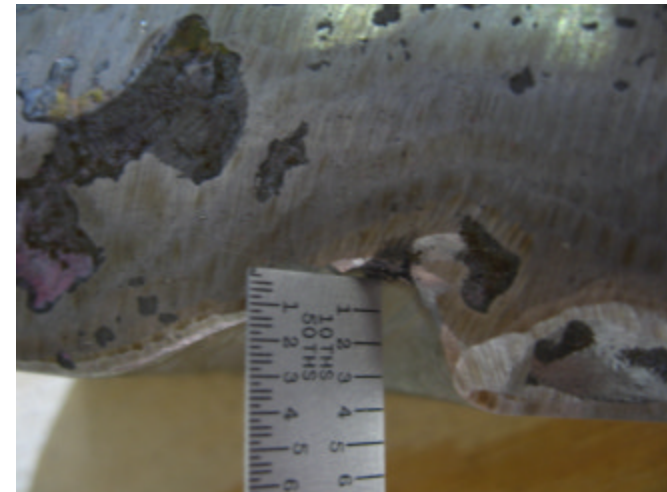
Tool Gouge on perimeter of Datum E flange, approximately 1" wide by .50" deep.
