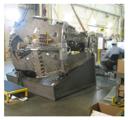
3.4.6 Lower the mating "B" coil into position.
