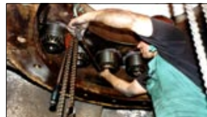
Overhead work is simplified with the low torque requirement on this Turbine Wheel to Shaft bolting. Galling and seizure is eliminated.
