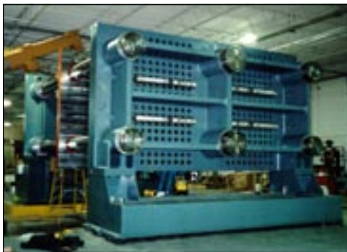
2,500 Ton Structural Foam Injection Molding Press. Installation was accomplished in 2 hours using hand tools!
