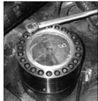
Armored Torquenut on large machinery. Recessed jackbolts can be helpful when there is flying debris or when more thread engagement is needed.
