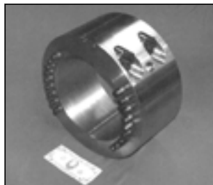
18" split nut used on aluminum extrusion press tie rods.
