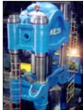
Press Anchorbolt on 2,000 Ton Hydraulic Press.
