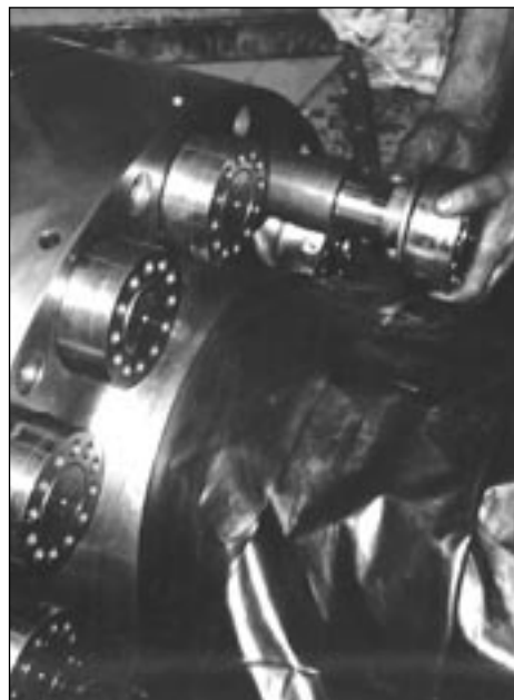
Large turbine/generator coupling. Installation 4 hours, removal 1 hour.
