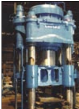
20" diameter Supernut™ Tensioners on a 5,000 Ton Forging Press.
