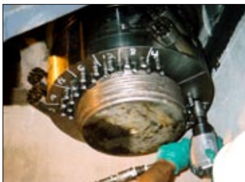
16-1/2" split nut on forging press columns.
