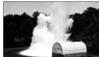
Superbolt tensioners passing shock qualifications at hull integrity levels at the HiTest Laboratories facility, Arvon, VA.
