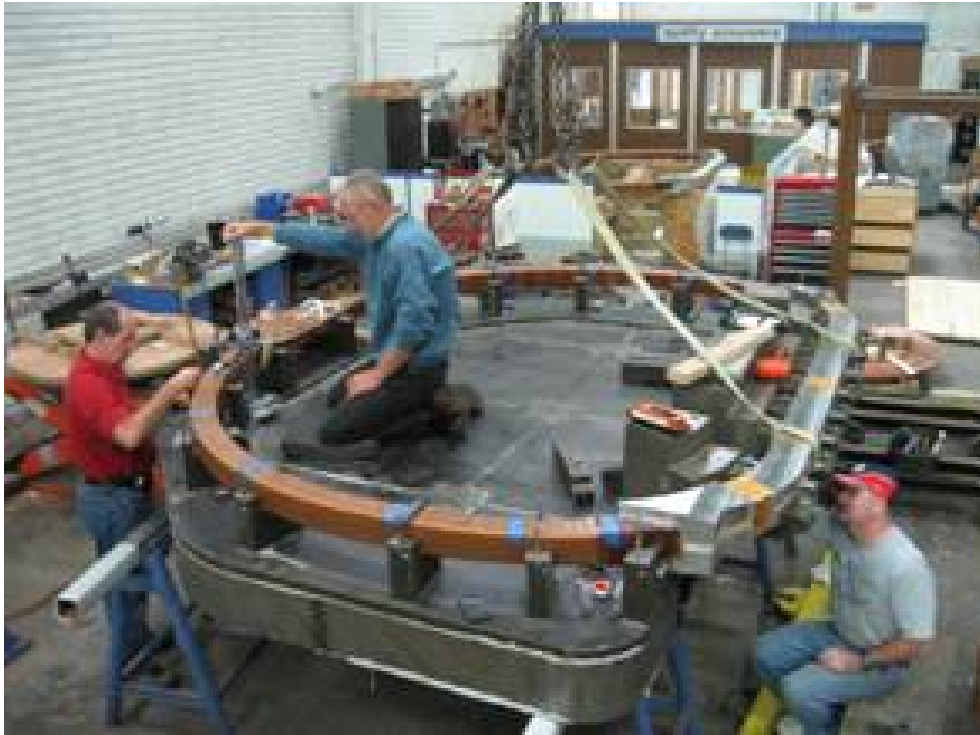
Figure 6: One of the 18 NCSX toroidal field coils fabricated by industry and delivered to PPPL.
