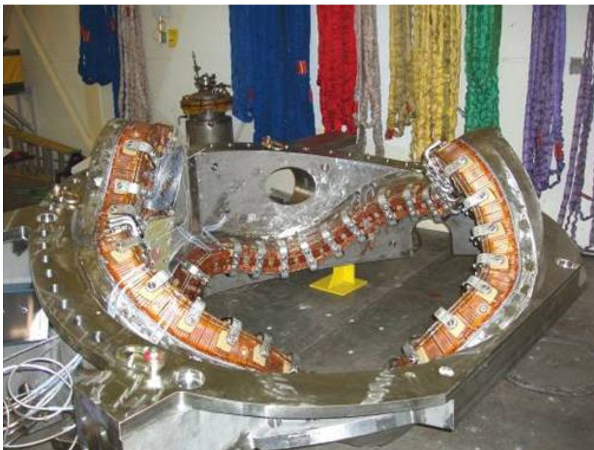
Figure 12: Modular coil after vacuum impregnation at PPPL.
