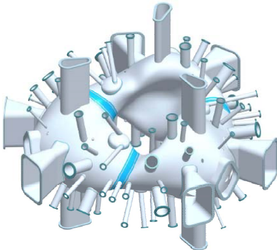
Figure 3: NCSX vacuum vessel design.
