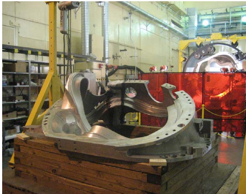
Figure 9: Modular coil winding form fabricated by industry and delivered to PPPL.
