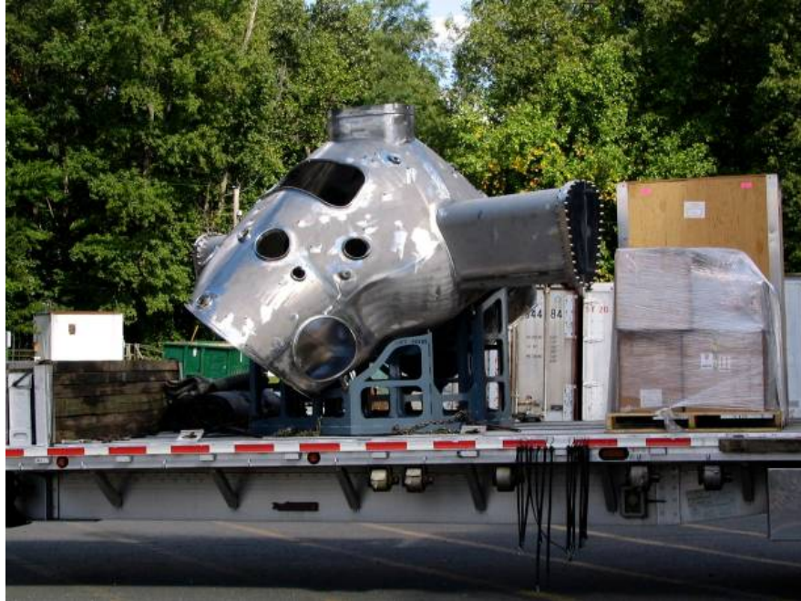
Figure 4: One of three NCSX vacuum vessel sectors fabricated by industry and delivered to PPPL.
