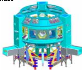
4. Interior mid-sections and upper/lower flat sections installed
