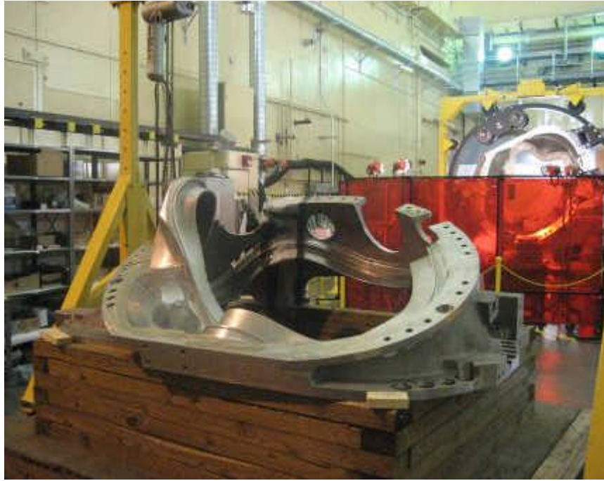
Figure 14: Modular coil winding form fabricated by industry and delivered to PPPL.
