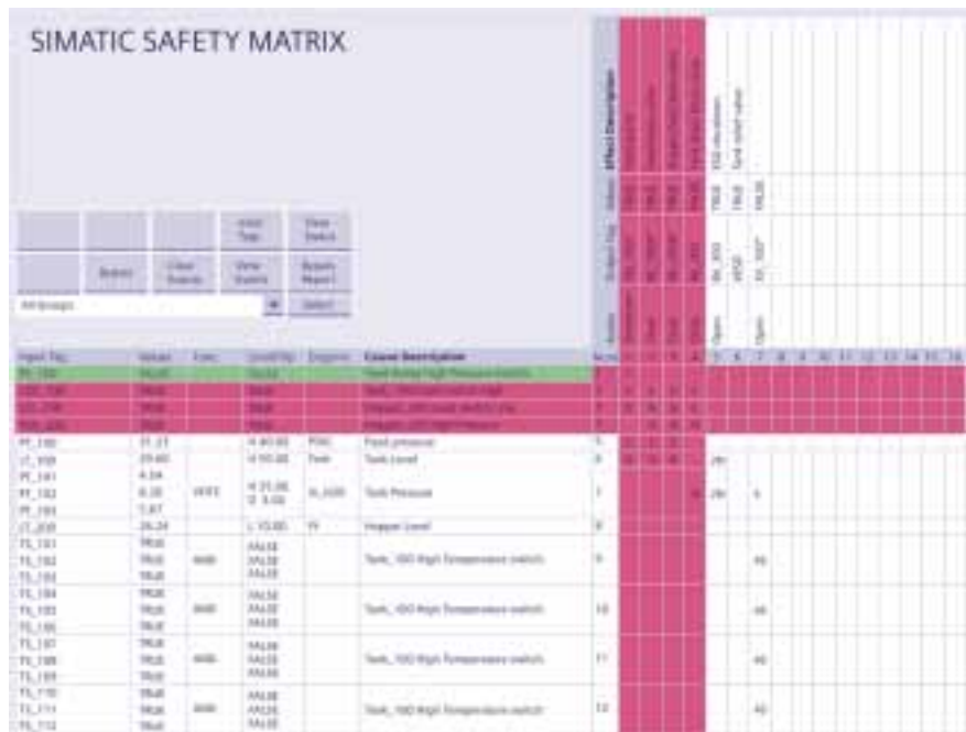
Fig. 7/5 Example of the SIMATIC Safety Matrix for S7-400FH
