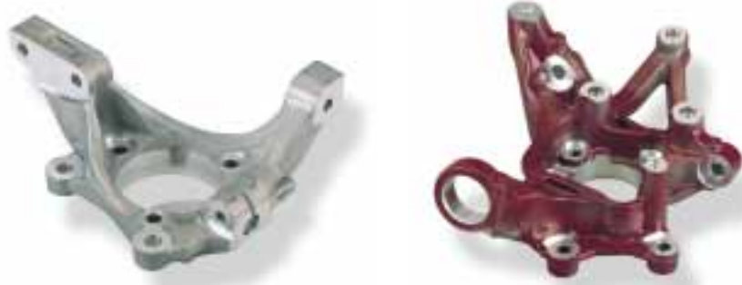
Aluminum reduces the weight of an automobile. In this particular case with Opel, these aluminum wheel hub carriers and pivot axes reduce the weight by 6.6 kg with respect to cast iron parts
