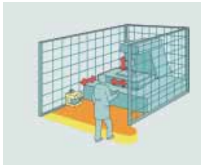
Fig. 6/13 Securing stationary dangerous areas
