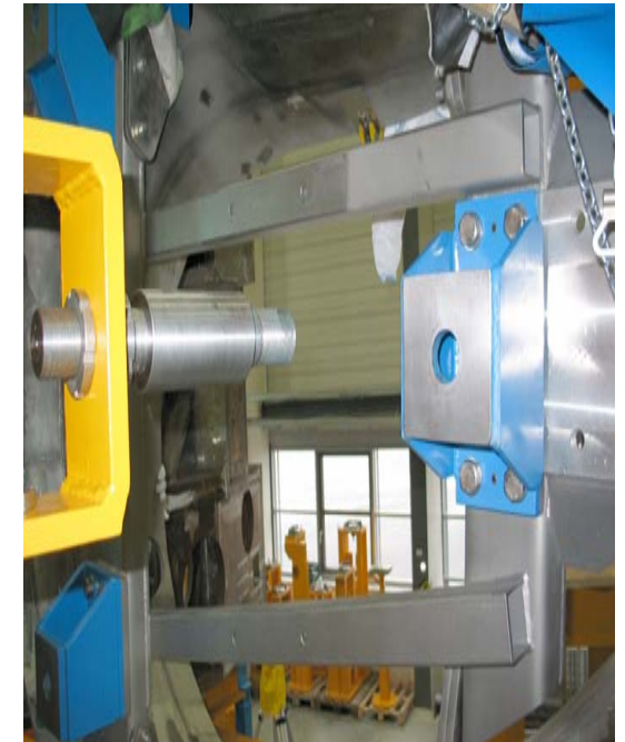
Figure 9: Real flange scenario between HS01-sector and a mechanical structure in stand I/B.
