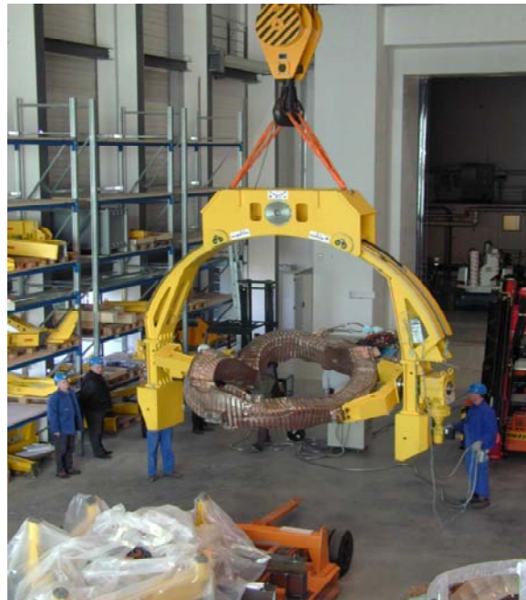
Figure 4: Load- and motiontests with SAE-1 and non-planar coil NPS1 in the IPP (2004)
