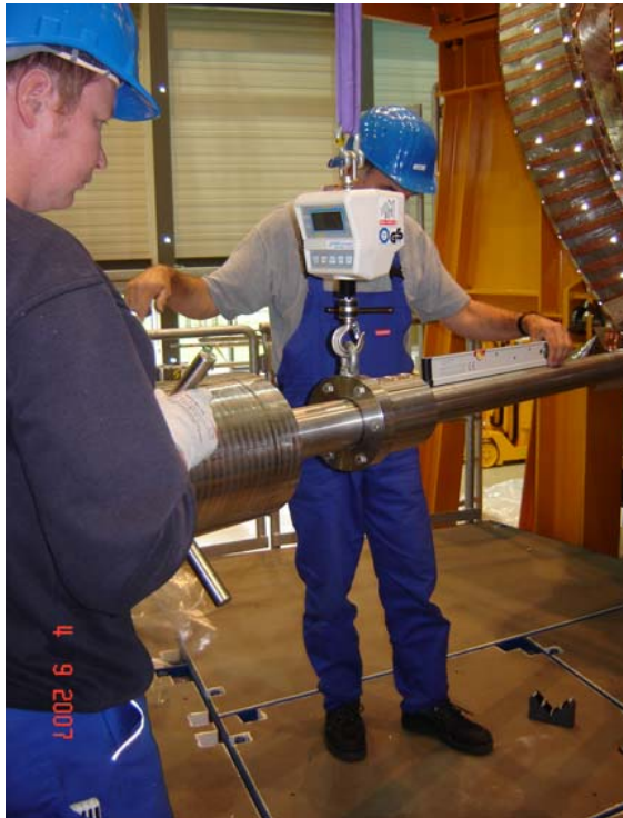
Figure 14: Assembly of the CSE for the connecting the coilsystem with central ring with bolts.
