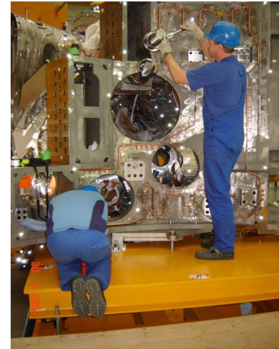
Figure 15: Set up test for the central ring- semi- module onto linear sliding frame. The weight for central ring- semi- modul is 7,2 tons.
