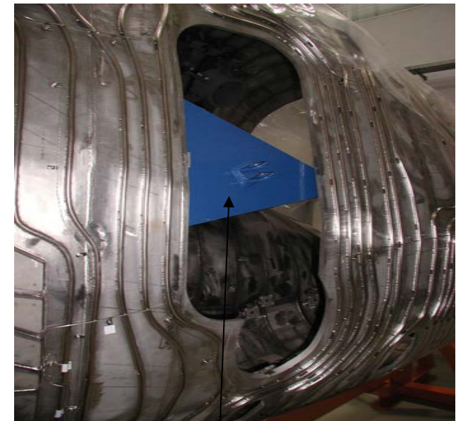
Figure 18: Plasma vessel sector 51HS02. Bearing flange solution (half-module- side) with fixation-point in a port at plasma vessel.
