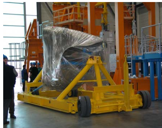
Figure 5: HS02- sector transport with a 150 kN- flatcar. The flatcar will be used for transport between neighbouring halls.
