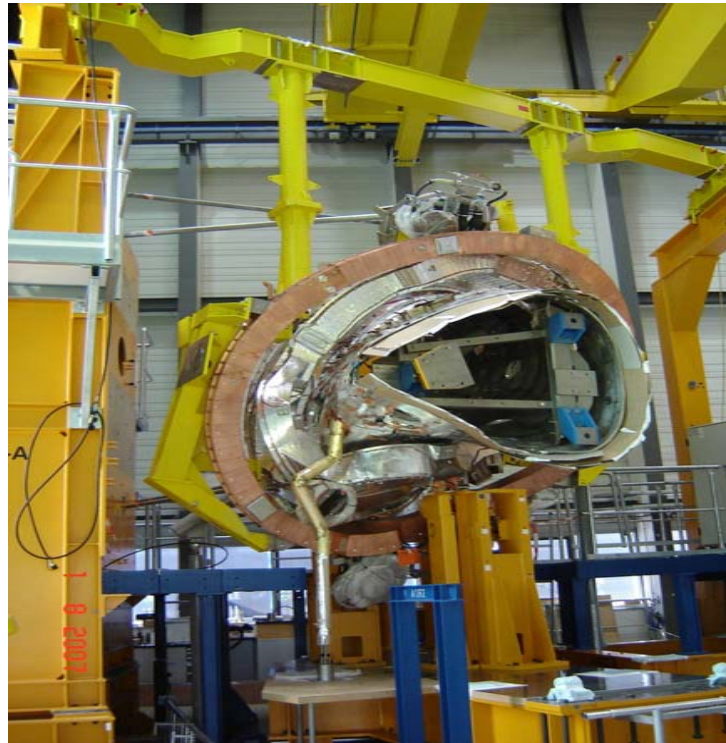
Figure 9: Interaction SAE-2, NPC4- Liftraverse and headover crane (2003). SAE-2-motion training with a blue test item (mass 6000 kg)
