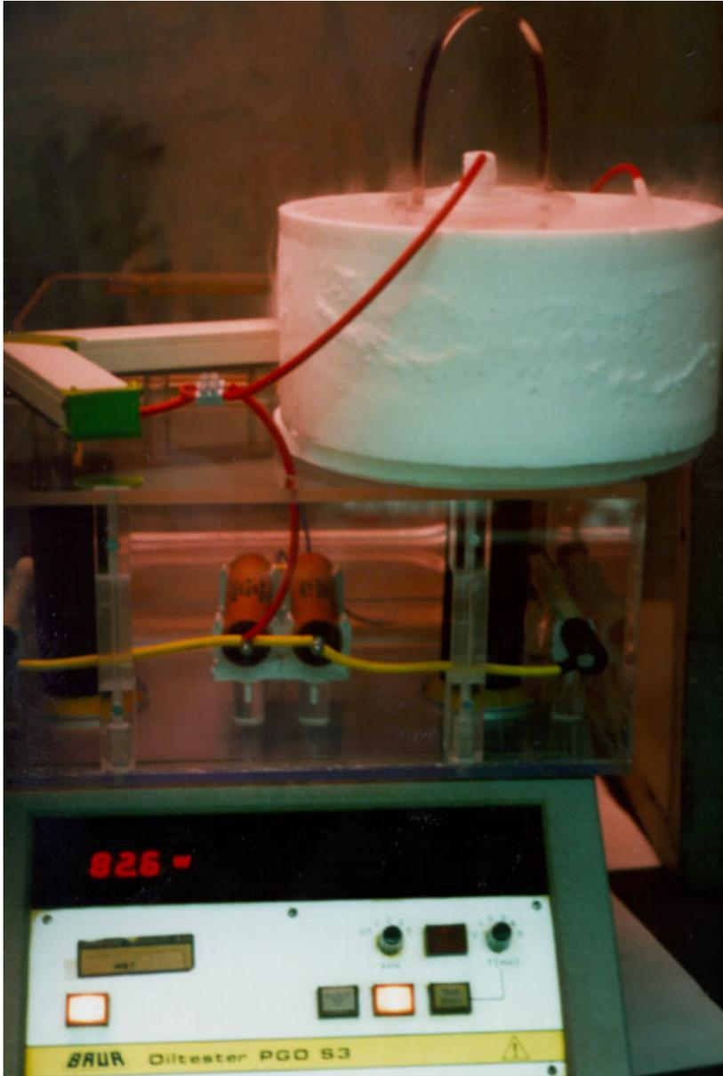
**Figure 11:** The measuring device in the liquid nitrogen container connected with the high voltage power supply.
