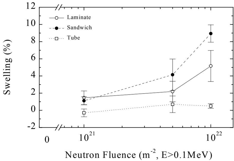
**Figure 7:** Swelling of the laminate, the sandwich, and the conductor insulation prototype sample (tube) after reactor irradiation.
