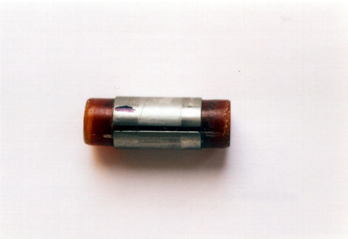
**Figure 4:** Photographs of the conductor insulation prototype sample (tube).
