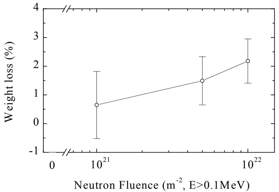
**Figure 8:** Weight loss of the laminate after reactor irradiation.
