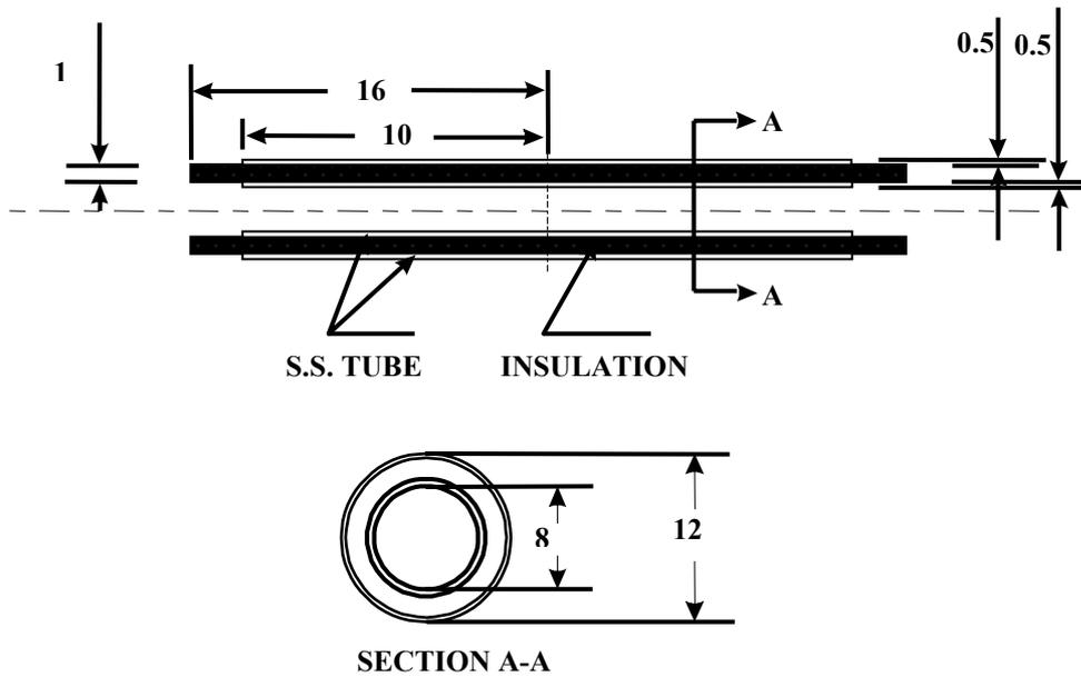
Figure 1: Insulator and insulator-metal sandwich sample.
