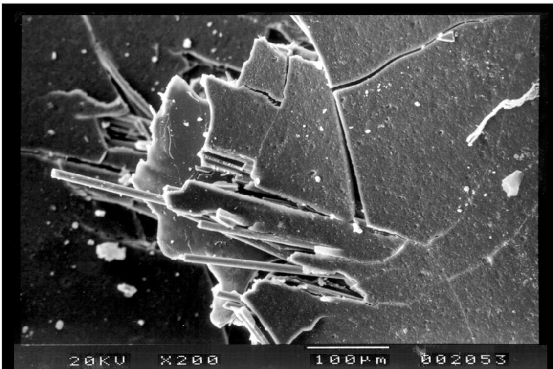
**Figure 13:** SEM photographs of the surface of the laminate following reactor irradiation to a neutron fluence of  $1 \times 10^{21} \text{ m}^{-2}$  ( $E > 0.1 \text{ MeV}$ ) and electrical breakdown at 77 K.
