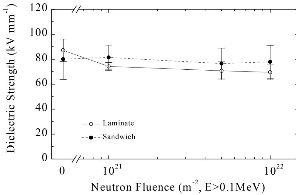
**Figure 12:** Dielectric strength of the laminate and of the sandwich as a function of the neutron fluence.
