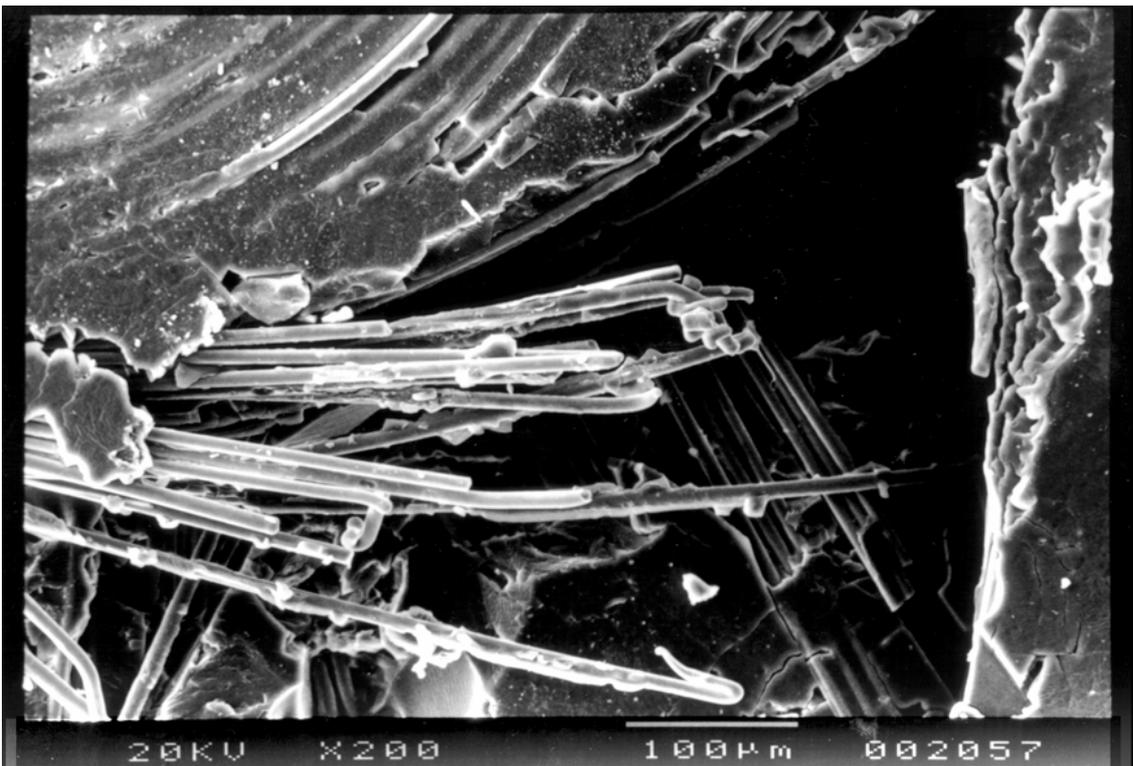
**Figure 15:** SEM photographs of the surface of the laminate following reactor irradiation to a neutron fluence of  $1 \times 10^{22} \text{ m}^{-2}$  ( $E > 0.1 \text{ MeV}$ ) and electrical breakdown at 77 K.
