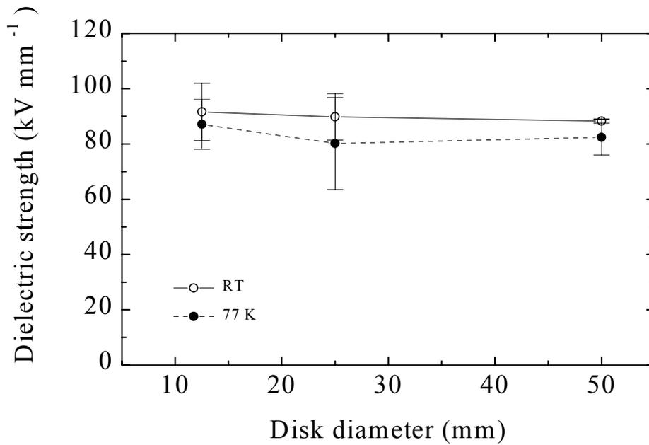
**Figure 10:** Scaling result on unirradiated disk shaped laminates.
