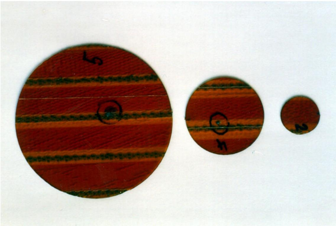
**Figure 9:** Photograph of the disk shaped laminates for scaling tests.
