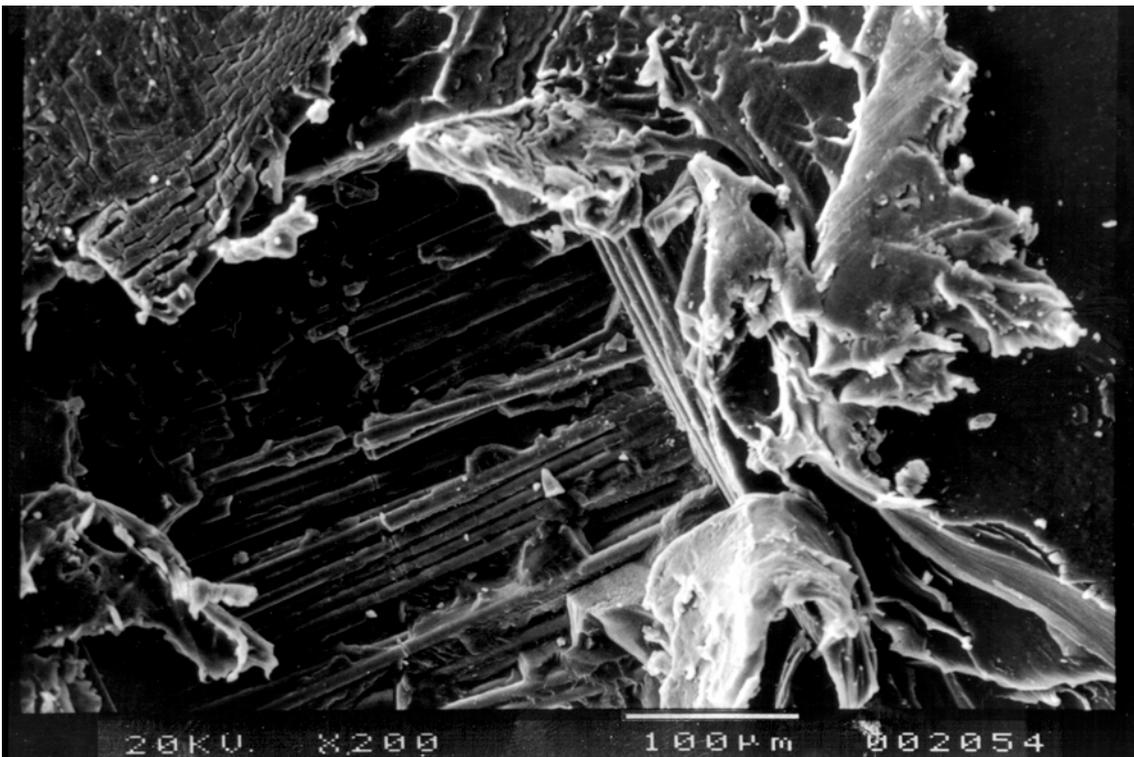
**Figure 14:** SEM photographs of the surface of the laminate following reactor irradiation to a neutron fluence of  $5 \times 10^{21} \text{ m}^{-2}$  ( $E > 0.1 \text{ MeV}$ ) and electrical breakdown at 77 K.
