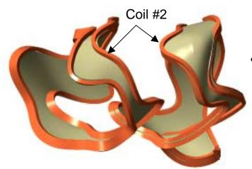
• Conformal shell segments with ½ coil wound into each end.
