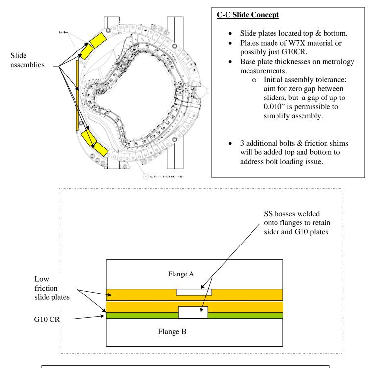
attachment scheme: weld 1" diameter pins onto both flanges (say, 2/slider). Insulate OD of pins with G10CR sleeves; slide plates and G10CR would have clearance holes to permit them to simply be "hung" on the pins.
