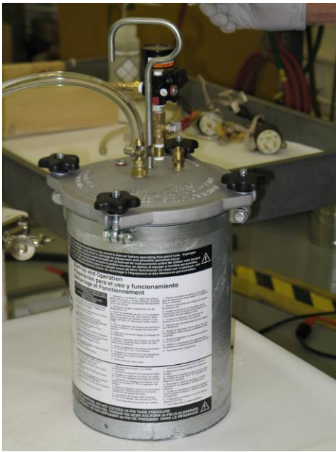
Paint pot used as vacuum chamber
