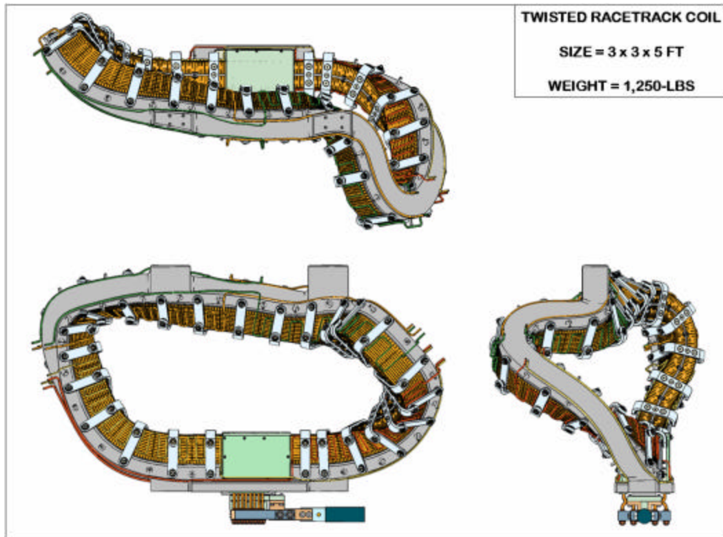
Figure 1-1 - Twisted Racetrack Coil Assembly
