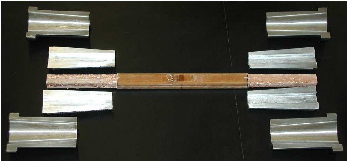
Figure 9. ISMC tension specimen, aluminum tension test angular grips, and stainless steel grip holders.
