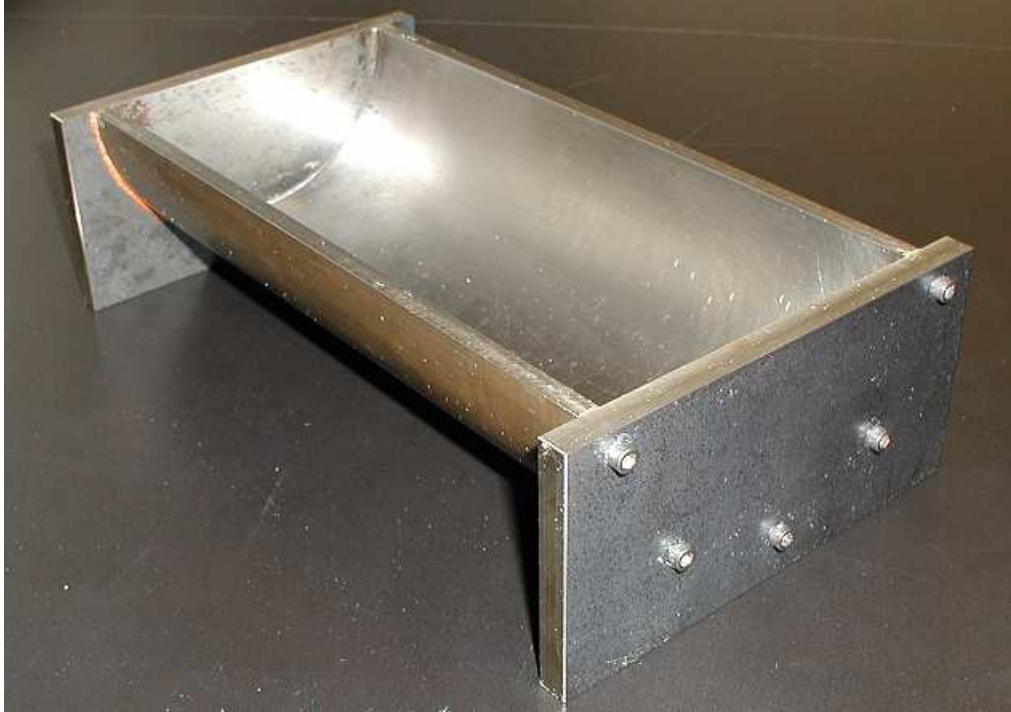
Figure 1. Steel mold used for cure shrinkage tests.
