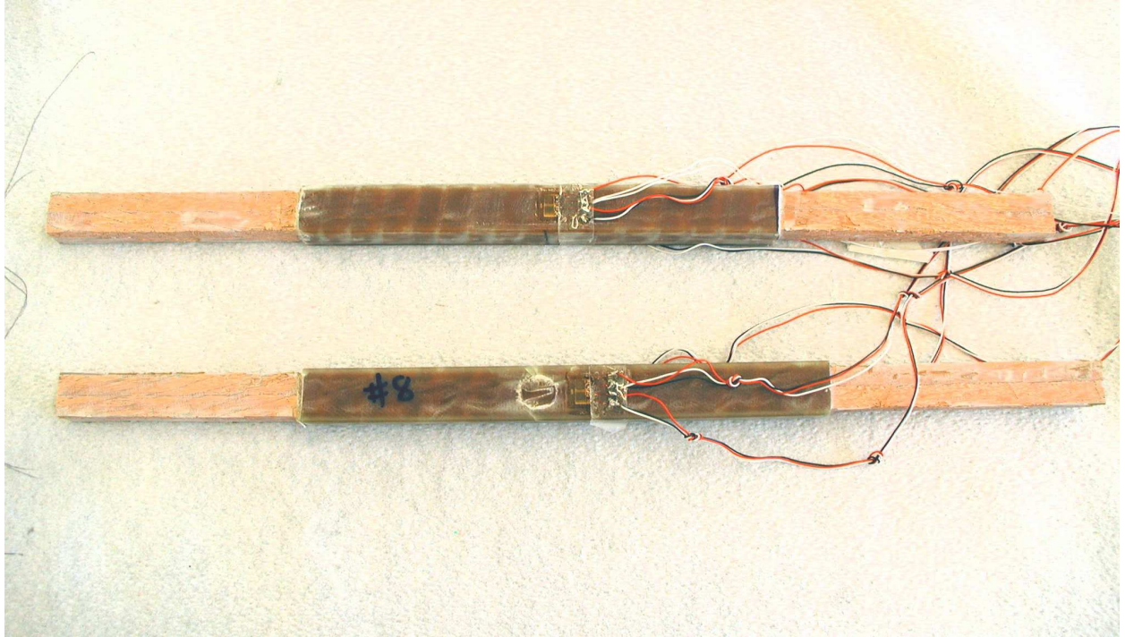
Figure 8. ISMC tension specimens with insulation removed from ends.
