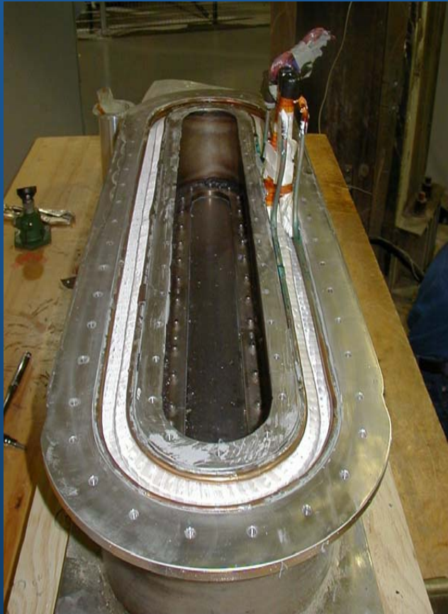
Epoxy impregnated Univ. of Tenn. Racetrack Coil
