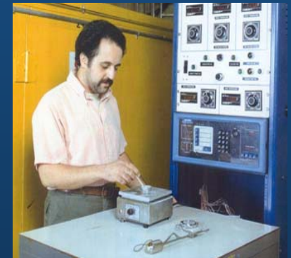
“Scrambled Egg” test to verify Gel temperature
