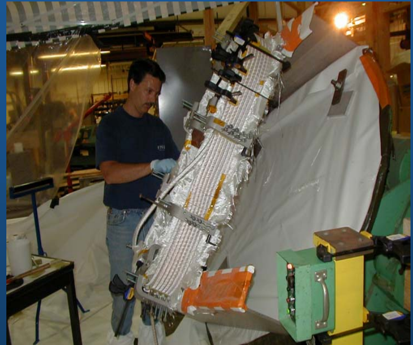
Wound and epoxy impregnated Racetrack Coil at PPPL
