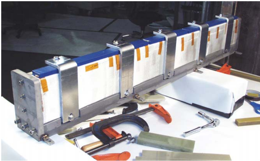
18 Insulated Turns in Position on Tee Section – Figure 5
