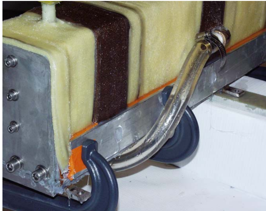
Edge View of Mold Ready for Oven and VPI Figure 10
