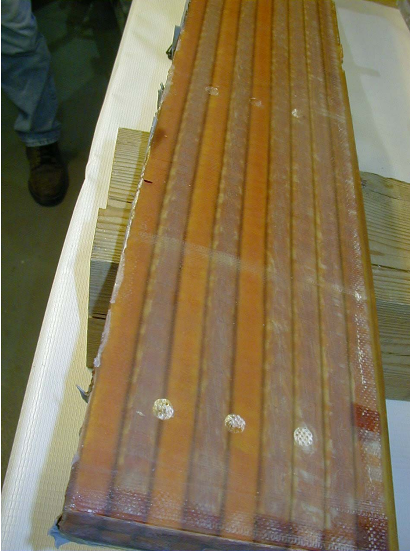
Vacuum Impregnated Bundle (18) turns from Tee Section- March 11, 2003 Figure 12
