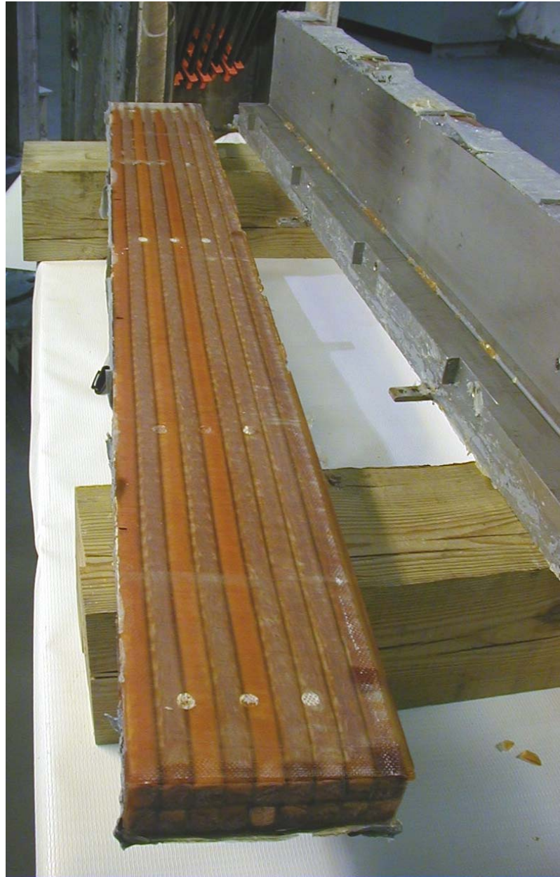
Vacuum Impregnated Bundle (18) turns from Tee Section- March 11, 2003 Figure 11
