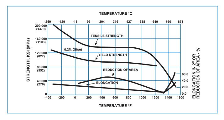
The aging reaction in Altemp A286 alloy may be conducted on either solution treated or solution treated and subsequently cold worked material. In the latter case, the aging reaction results in a further increase in strength and hardness in comparison to solution treatment and direct age. This tendency is balanced by the tendency of higher aging temperatures to relieve some of the effects of the cold working operations.
