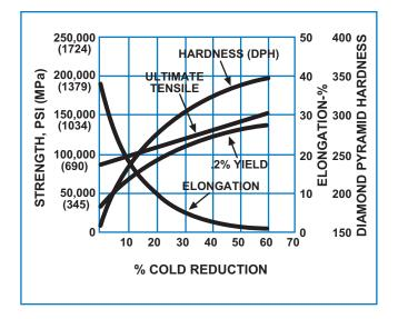
Intermediate anneals at 1800°F (982°C) can be employed to soften the material if the cold deformation is extensive.
