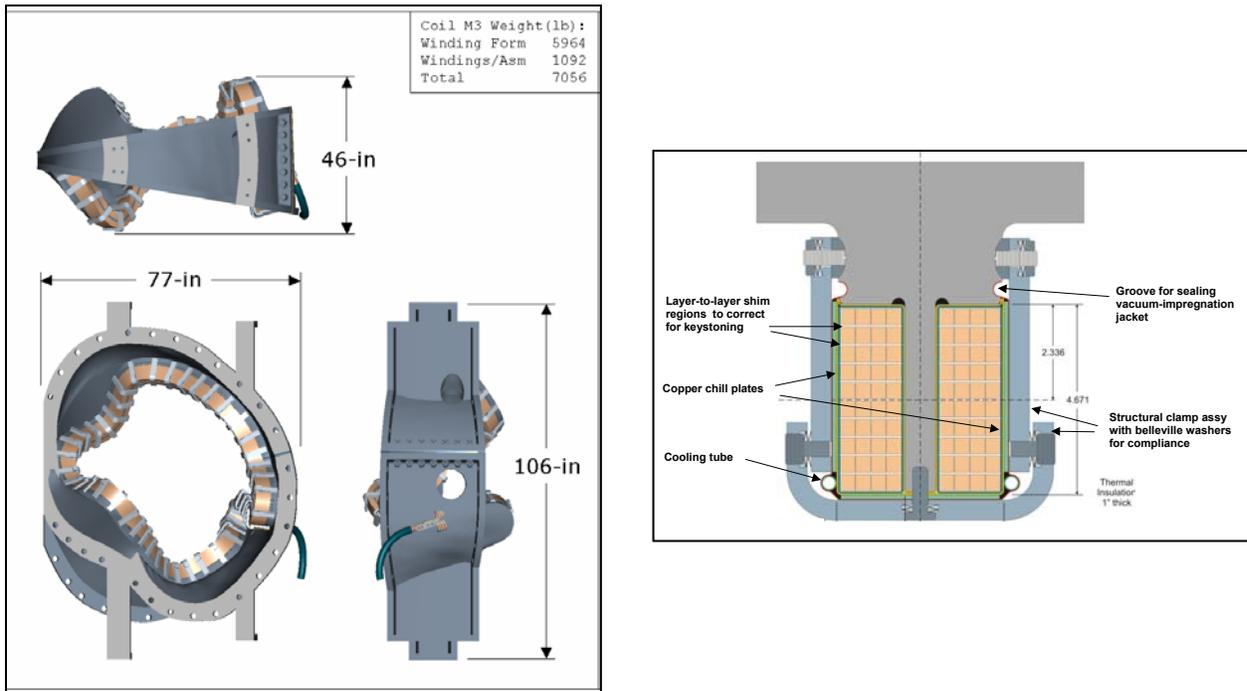
**Figure 3.1-1 Details of a Typical Winding Form**
